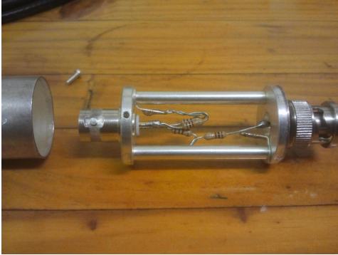
Figure 3.5: Resistive matching termination
