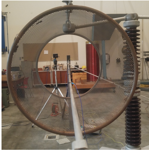
Figure 3.2: Corona test cage
