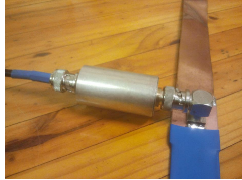
Figure 3.6: 250/50 \text{ } \Omega Termination
