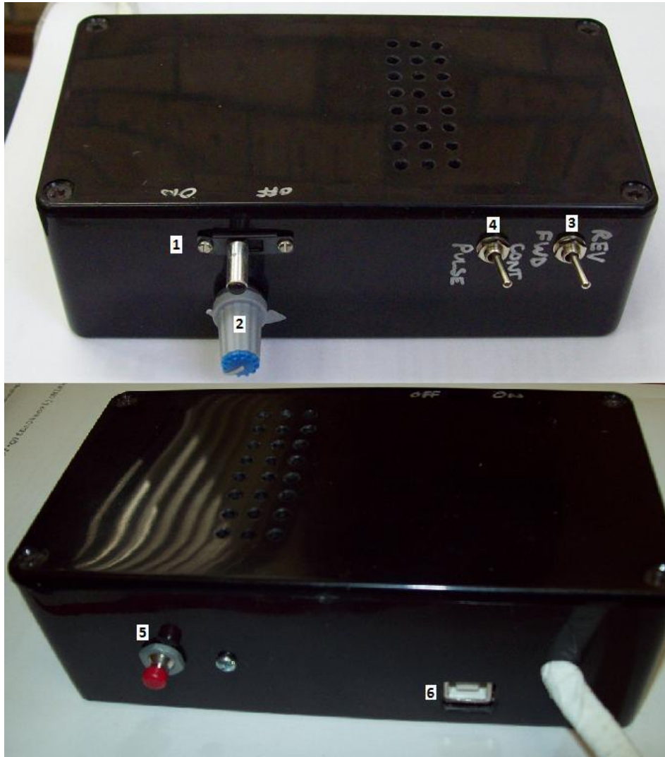
Figure D.2: Motor hand control. The respective items on the control are: (1) on-off switch; (2) speed control; (3) motor direction; (4) internal/external control; (5) pulse button; (6) USB connection point.
