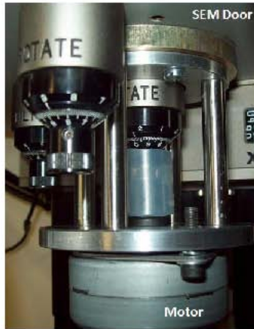
Figure 4.18: SEM-Motor coupling arrangement. An aluminium bracket and brass spacer mount the motor on to the door at the correct distance. Silicon tubing transmits motion between the motor and SEM shafts, both of which have dials attached for shaft location reasons.
