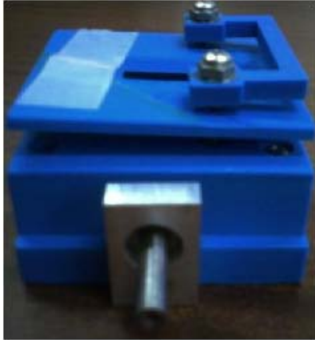
Figure 4.9: Full view of a previous pivot-type rig. The top plate rests on the base through a pivot located under the left side of the plate, as seen in this picture. On the right there is a loading arm which is drawn down and depresses the plate on to the specimen resting underneath.
