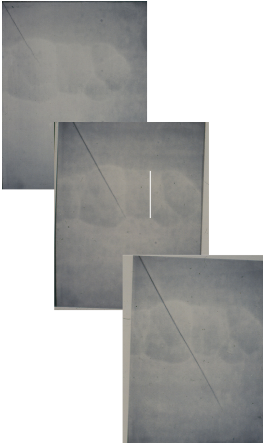
Figure 3.17: Crack propagation in glass at different loading stages; glass etched with hydrofluoric acid as a viewing aid. Crack propagating from top left, in series, to bottom right. The neck of the etch pit highlighted in the second image is of the order of a micron, shown by the micron bar. [50]
