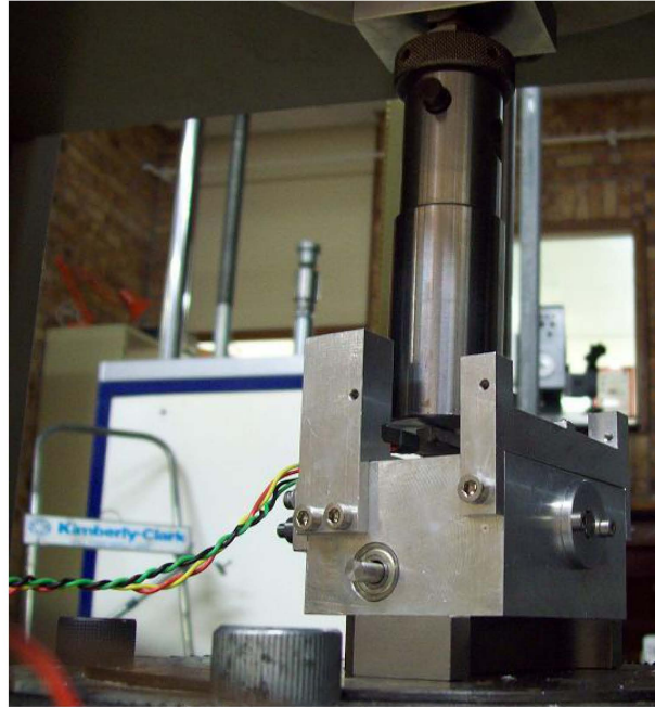
Figure 5.3: Setup for the evaluation of the strain bars. A cylindrical grip is attached to the crosshead of the Zwick tensile/compression machine, and brought to bear down on the front specimen support through which load is transferred to the strain bar beneath. The bar is just visible resting inside one of its support grooves. Also visible are the wires connecting the gauges to the strain indicator.
