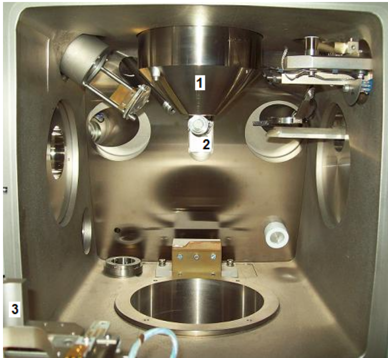
Figure 4.2: Photograph showing the interior of the SEM specimen chamber. The electron beam aperture (1) protrudes from the ceiling centre, with the secondary electron detector (2) protruding from the back wall. The stage arrangement, which is fitted to the open door, is just visible in the bottom left (3).
