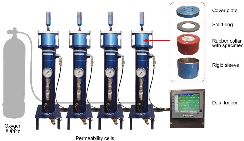
Figure 3-7 OPI test set-up.
