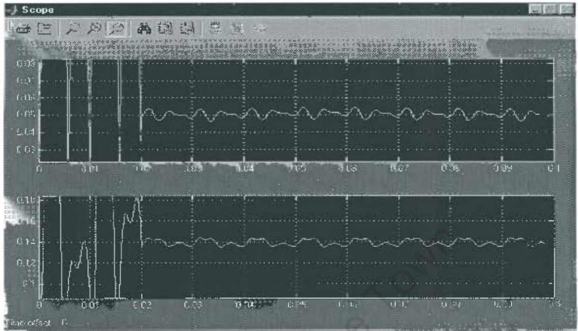
Fig: 7.23 Magnitude of the 5th order voltage and current harmonics in a saturated core
