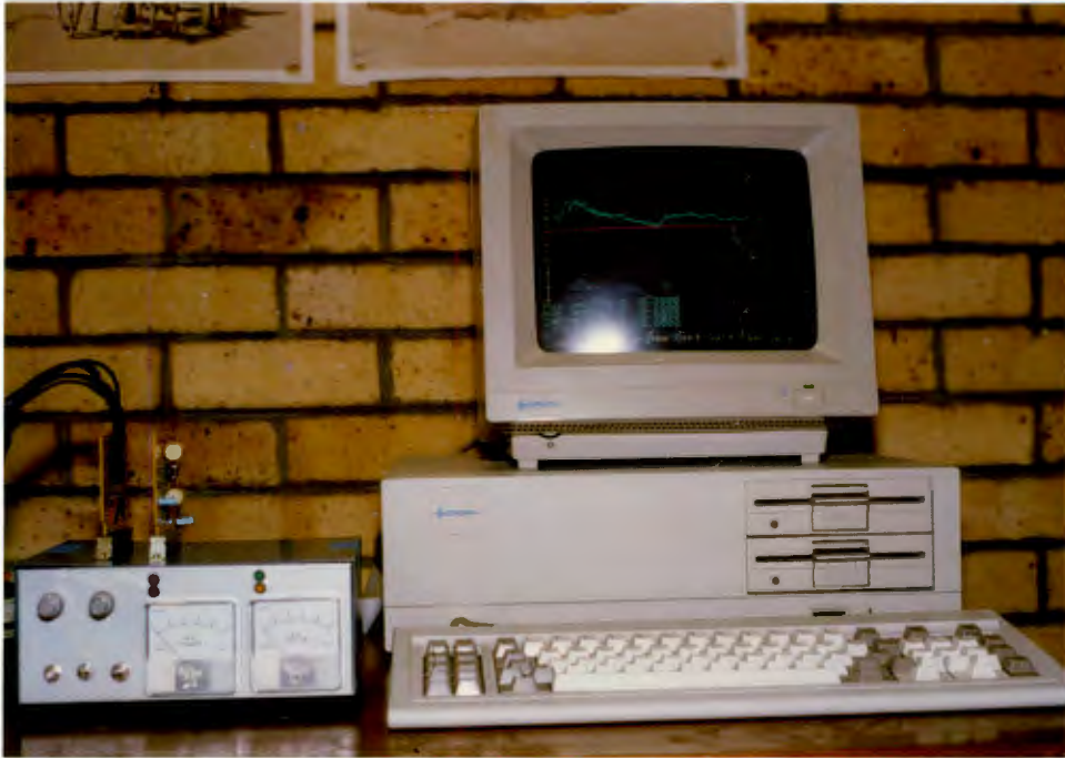
A SIMULATION INVOLVING GAUSSIAN NOISE IN PROGRESS ON A SPERRY PC, WITH THE USER INTERFACE CONNECTED ON THE LEFT
