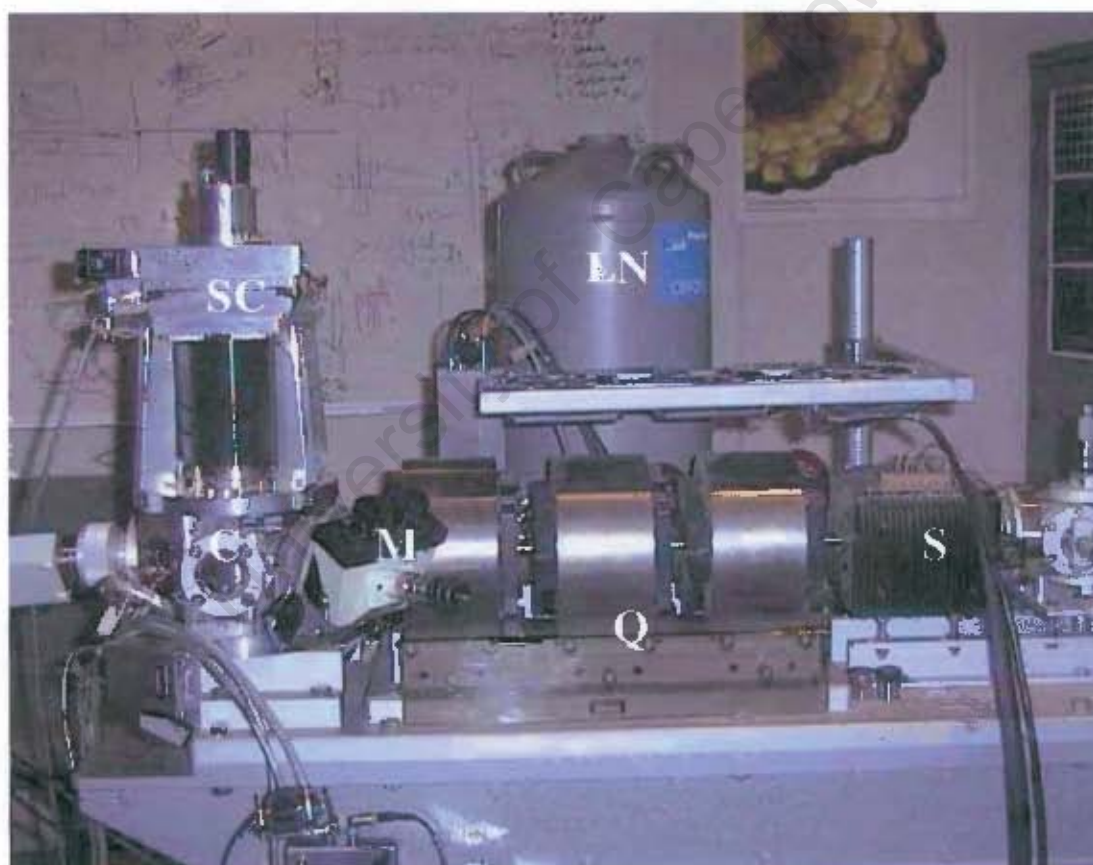
Figure (7.4) Photograph showing the layout of the nuclear microprobe (NMP) system, H is the halo slits, S is the scanning coils used to position the beam probe on the specimen surface, LN is the container for cooling the Si(Li) detector used in the detection of X-rays, Q the set of quadrupole lenses, used in the focusing of the beam, M the optical microscope for viewing the specimens, C is the nuclear microprobe scattering chamber and SC is the sample change mechanism.
