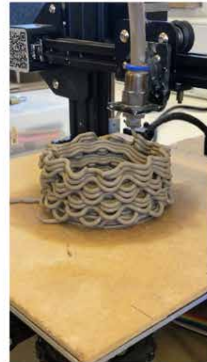
Image showing the result of the digital model being printed and how gravity influences the design.
