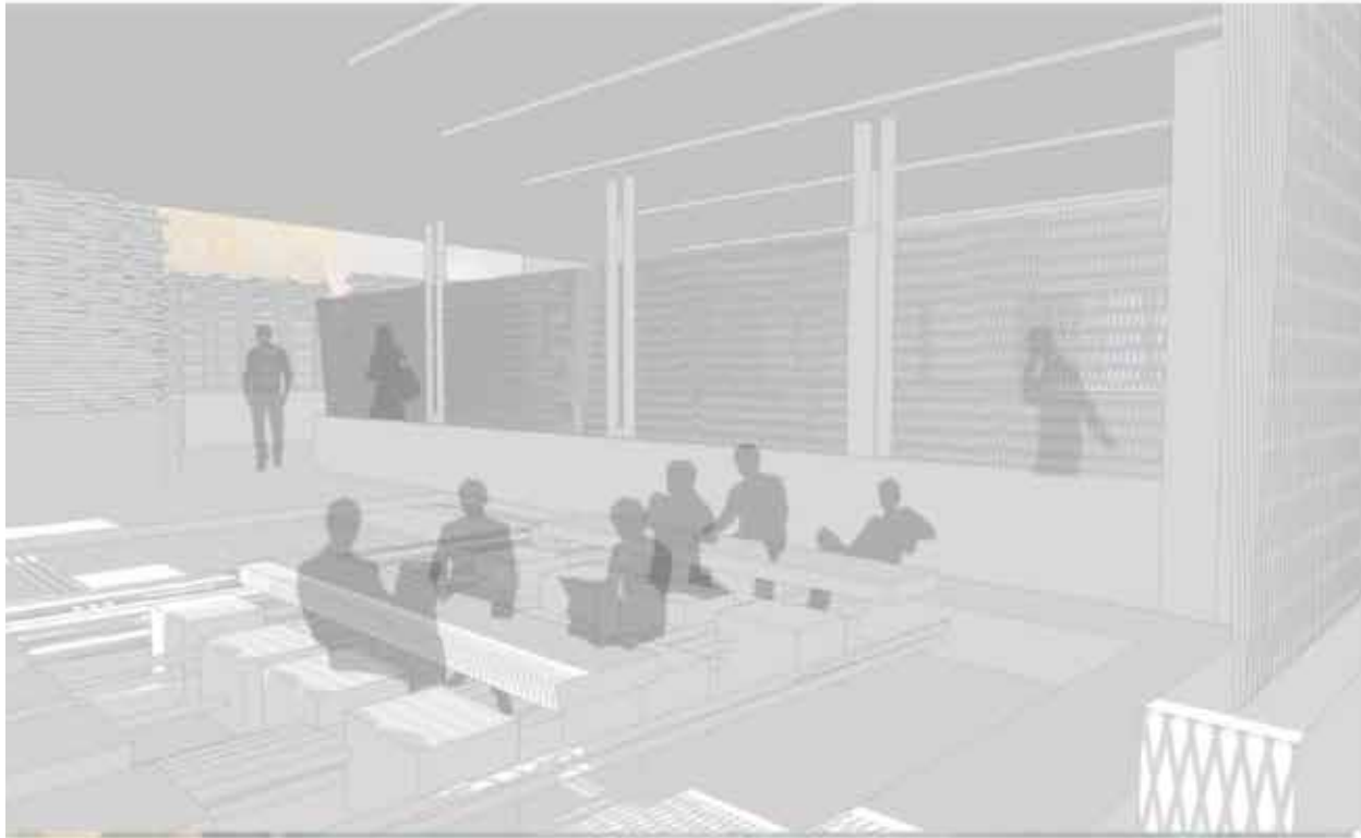
The layers of 3D printed mud walls add to thermal mass while the woven screen ventilate the space.
