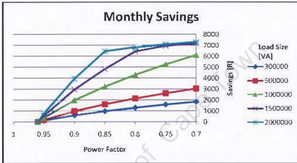
Figure 39: Graph - Monthly Savings Due to Power Factor Correction Versus Power Factor
