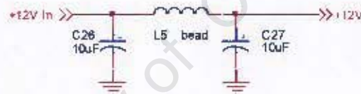
Figure 47: Schematic - LC Filtering of 12V Power Signal
