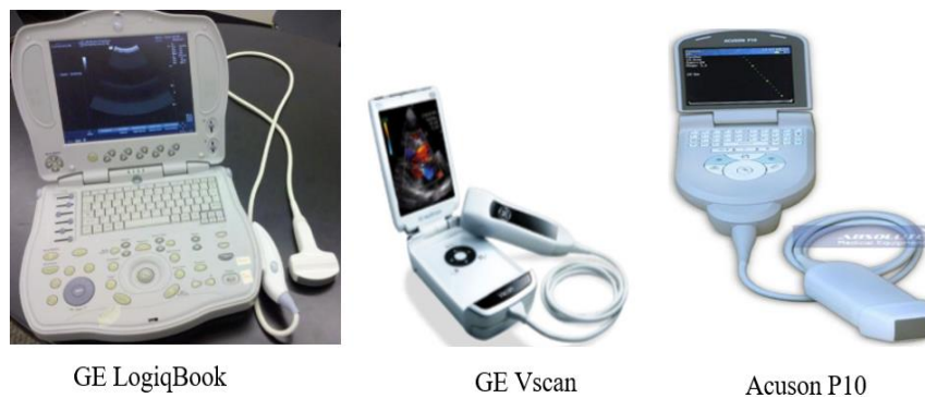
Figure 5: Conventional portable ultrasound systems with probe hardwired onto the processing unit; GE Logiq Book and GE Vscan from (GE Healthcare) and Acuson P10 (Healthineers, 2019).
