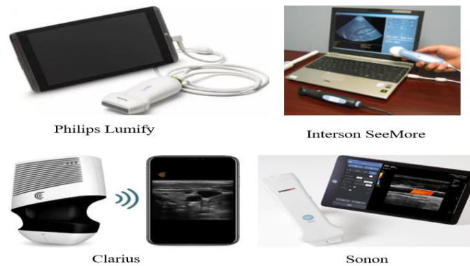
Figure 6: Mobile-based portable ultrasound systems with flexible probes; Philips Lumify from (Philips Lumify, 2019a), IntersonSeeMore from (Interson, 2019), Clarius from (Clarius Mobile health, 2018)and Sonon from (Healcerion, 2017).
