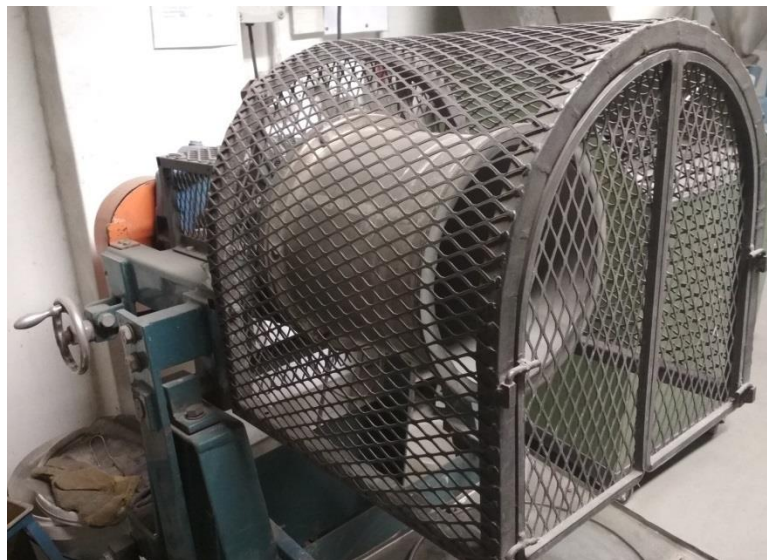
Figure 3-7: The 0.3 m diameter laboratory tumbling mill used for the test work.
