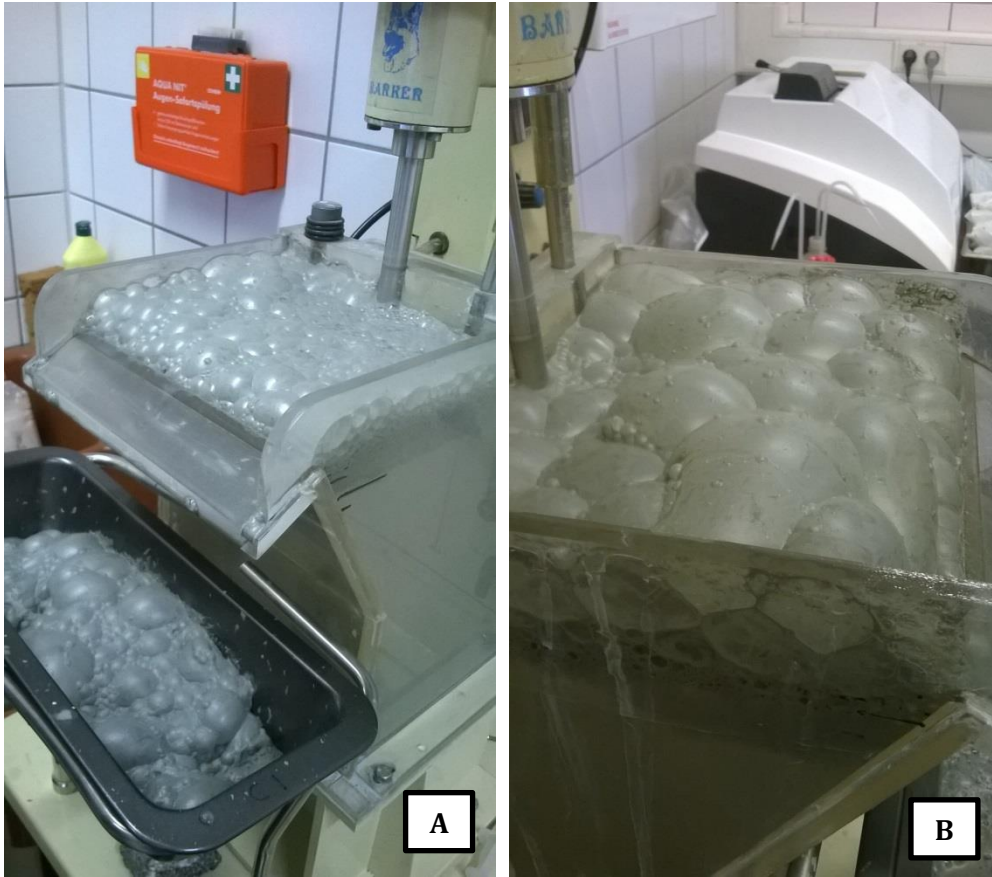
Figure 5-35: Pictures indicating the differences in the froth collected during the first minute of flotation for products of P_{80} 75 \mu\text{m} generated at a dam ring height of 7 mm at grinding pressures of 600 [A] and 800 [B] \text{kN/m}^2 .
