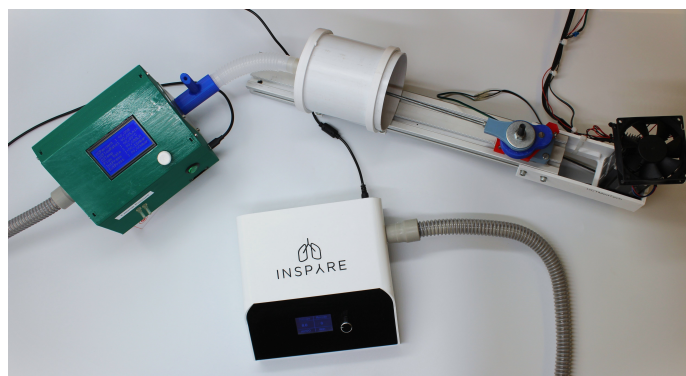
Figure 48: Dynamic Pressure Test Setup
