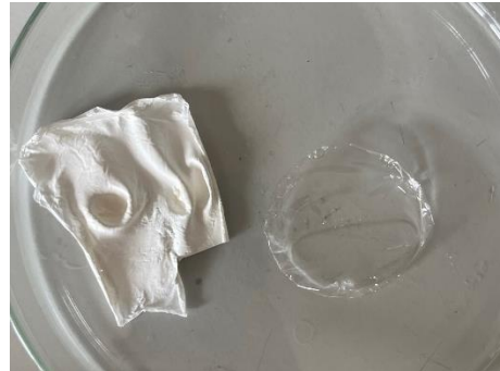
Figure 4-16: Electrospun & Cast materials post curing
