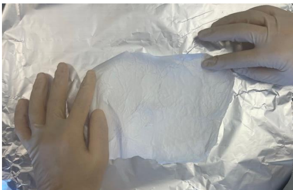
Figure 4-14: Electrospun mat after 4 hours
