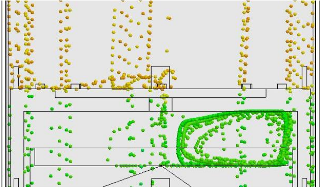
Figure 4-2: Particle bounce due to 'step down' design
