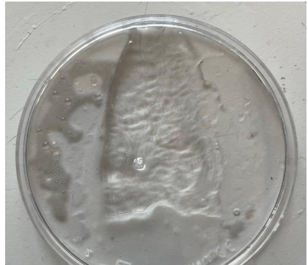
Figure 4-20: Electrospun mat after 12 hours in water
