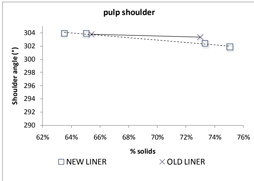
Figure 4.29(a) Pulp shoulder angles obtained from surveys with old and new liner conditions
