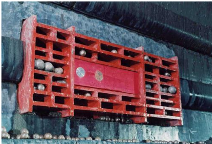
Figure 3.5 Specialised liner housing the beam with sensors of the Sensomag unit at Waterval UG2 Concentrator
