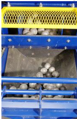
Figure 3.8 Detail of the smaller ball loading bin on the Magoload unit
