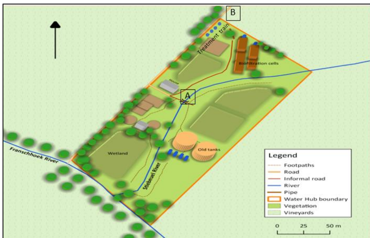
Figure 1. 2: Detailed overview of the Water Hub showing the biofiltration cells in relation to the Stiebeuel River, source: (Fell, 2017).
