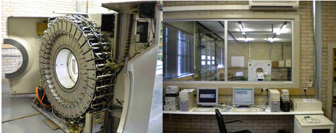
Figure 9: The “EXACT 3D” HR++ PET camera and control room at PEPT Cape Town laboratory [27].
