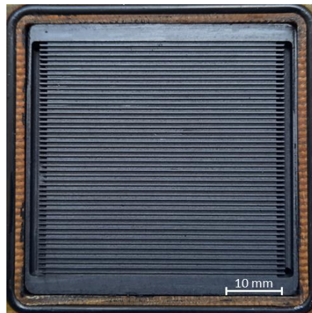
Figure A.1: Baltic straight parallel channel graphite flowfield used at the anode and cathode for all GDL configurations (land width = 0.3 mm, channel width = 0.6 mm, channel depth = 0.6 mm).
