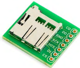
Figure 4.8 MicroSD Break out board. Taken from [54]
