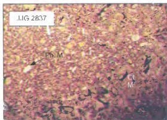
JIG 2837; Clewer Dyke. FOV ~20mm. Macrocrystic. Olivine macrocrysts are completely serpentinised and the majority are concentrated into one band. Groundmass consists primarily of phlogopite with lesser calcite and olivine.
