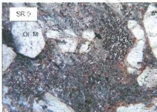
SR 9; Muil Dyke. FOV ~30mm. Euhedral to subhedral olivine macrocrysts are replaced by calcite, with serpentine along fractures. The groundmass is acicular and fine-grained, with a flow texture which bends around the macrocrysts.
