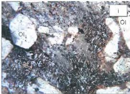
i) Typical appearance of the Muil dyke, showing euhedral or subhedral altered olivine macrocrysts and phenocrysts in a groundmass of needle-like phlogopite and diopside. FOV approx. 30mm.
