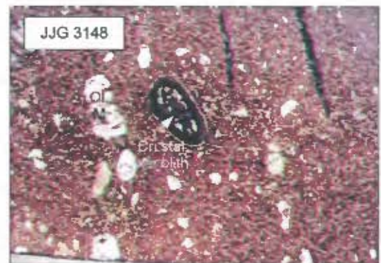
JJG 3148; South Fissure . FOV ~20mm. Olivine macrocrysts are completely replaced by calcite. The groundmass consists predominantly of phlogopite. A large crustal xenolith is present. The sample becomes more aphanitic towards the top right corner, close to the dyke margin.
