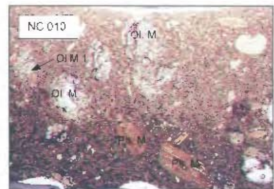
NC 010; Main Dyke. FOV ~20mm. Olivine macrocrysts are completely replaced by calcite, with some replacement by phlogopite of OL M 1. Phlogopite macrocrysts are highly strained. Groundmass is predominantly phlogopite.
