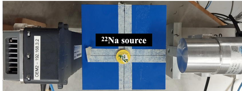
Figure 6.3.3: A photograph of the coincidence timing experimental setup of the Polaris and the 2'' \times 2'' \text{LaBr}_3:\text{Ce} detector with a low activity 13.80(138) kBq ^{22}\text{Na} source placed (0,0,10) cm from each detector face.
