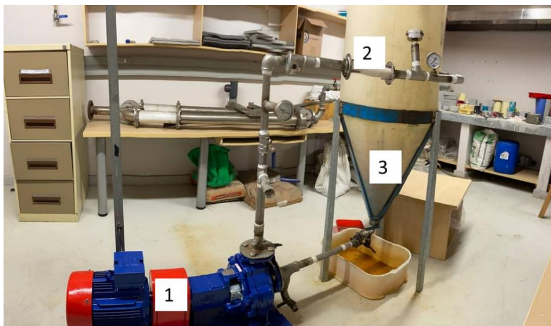
Figure 10: A simple schematic of the University of the Western Cape pilot cavitation system: (1) pump; (2) cavitation device; (3) solution tank.
