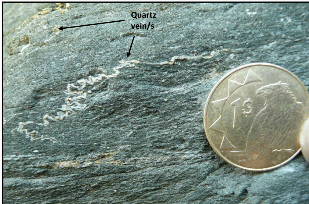
Figure 18: Outcrop of metamafic specimen MA-44. The rock is very fine- to fine-grained and grey - green in colour. Very thin quartz veins are observed. The coin for scale is 2.3 cm across.
