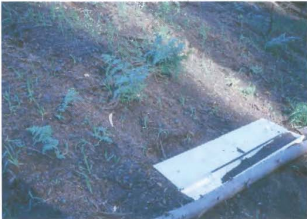
Figure 3.8: One-meter long gutters placed on all 20 plots at the FB site.
