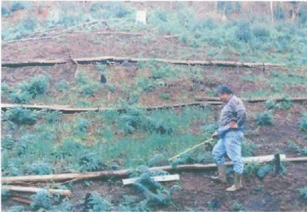
Figure 3.6. Three logs placed horizontally across the plots in the catchment that was “felled and burned”, as an additional stabilization technique.
