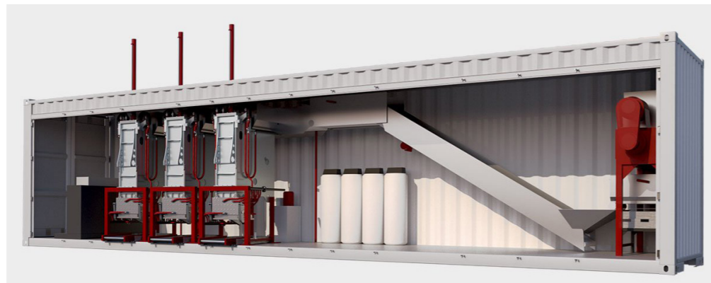
Fig. 55 - Blocker system. Plastic is fed into the system from the right, transported to the blockers which compress the ByBlocks (ByFusion, n.d.)
