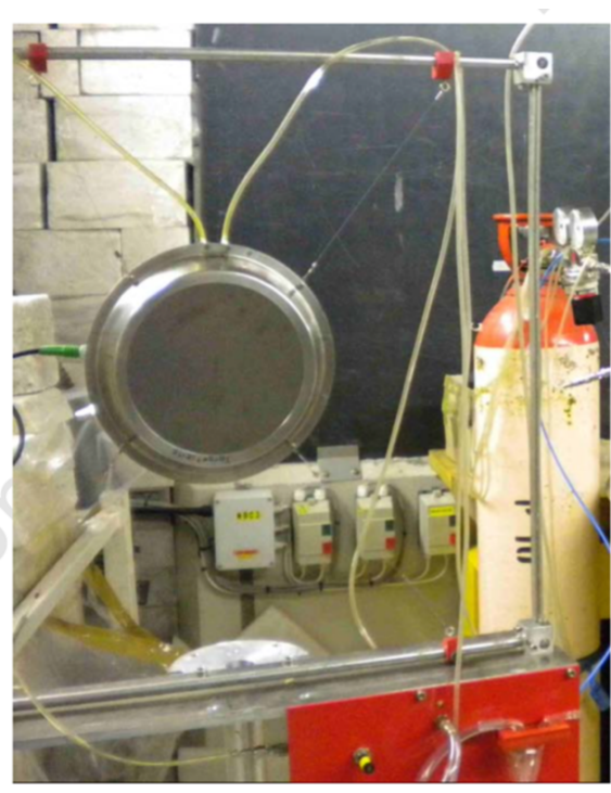
Figure 4.19: The ^{238}\text{U} FC in the D-line experimental vault.
