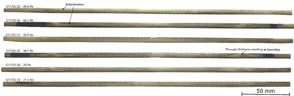
Figure 8-15: Cross-sectional photographs of blast tested Glass 17/Super Sap panels
