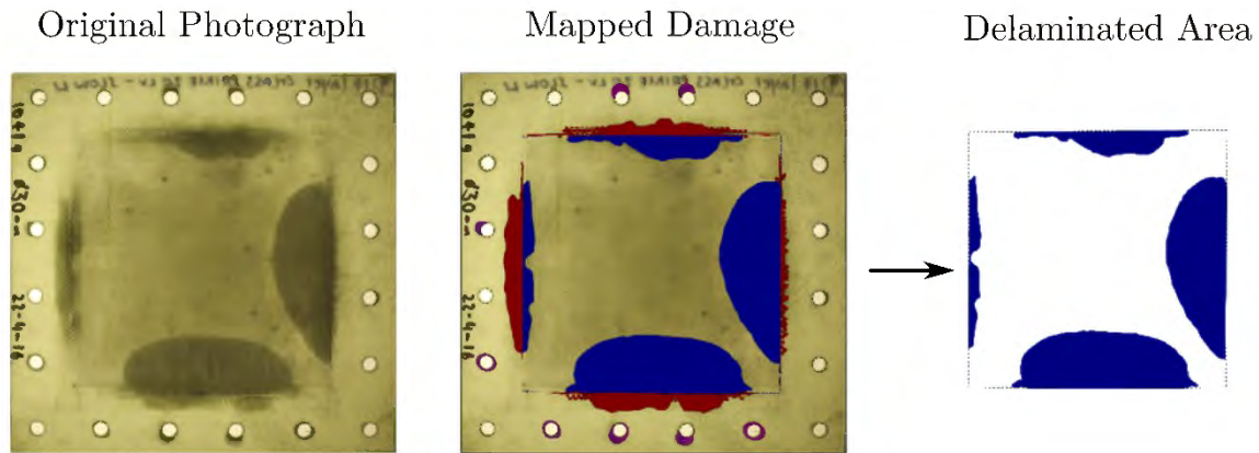
Figure 9-2: Photographs of G17/P20-9, using a lightbox, illustrating the mapped damage and the delaminated sections in the exposed area(blue)
