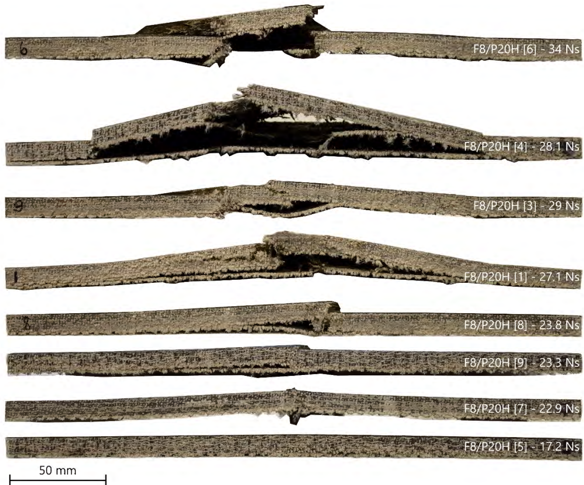
Figure 8-31: Cross section photographs for blast tested hand lay-up Flax/Prime 20LV panels
