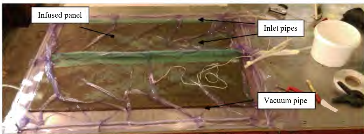
Figure 5-4: Photograph of an infused natural fibre composite on a flat moulding surface
