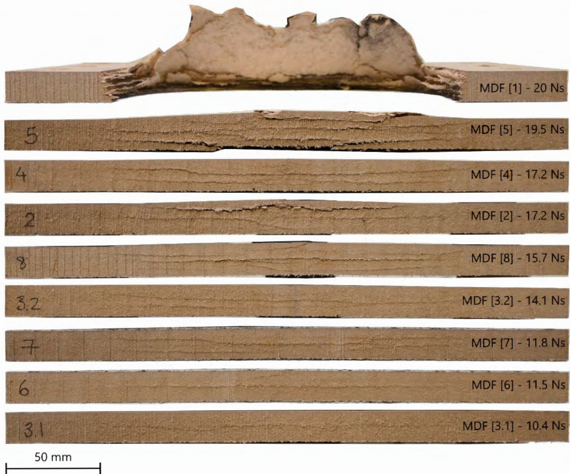
Figure 8-21: Cross section photographs for blast tested Supawood panels
