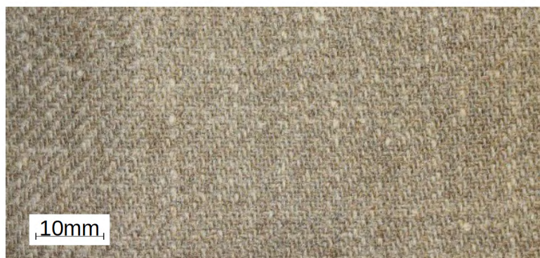
Figure 3-2: Photograph of twill 550 g/m 2 flax fabric
