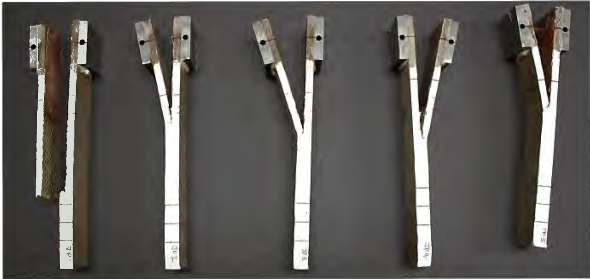
Figure 6-25: Photograph of broken DCB tested jute fibre reinforced composite specimens
