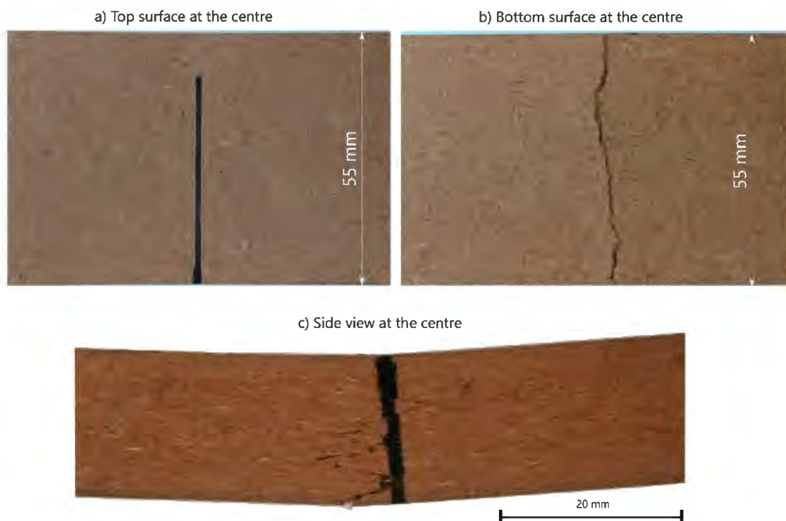
Figure 6-4: Photographs of the central region of a Supawood bend specimen after testing
