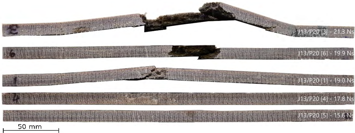
Figure 8-40: Cross section photographs for blast tested jute fibre reinforced panels
