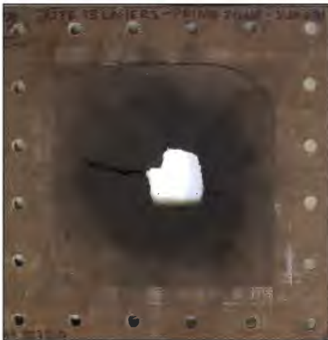
Figure F-2: Front and back surfaces of different blast tested Jute 13/Super Sap panels subjected to an impulse above 19.5 Ns (with no crack tracings)
