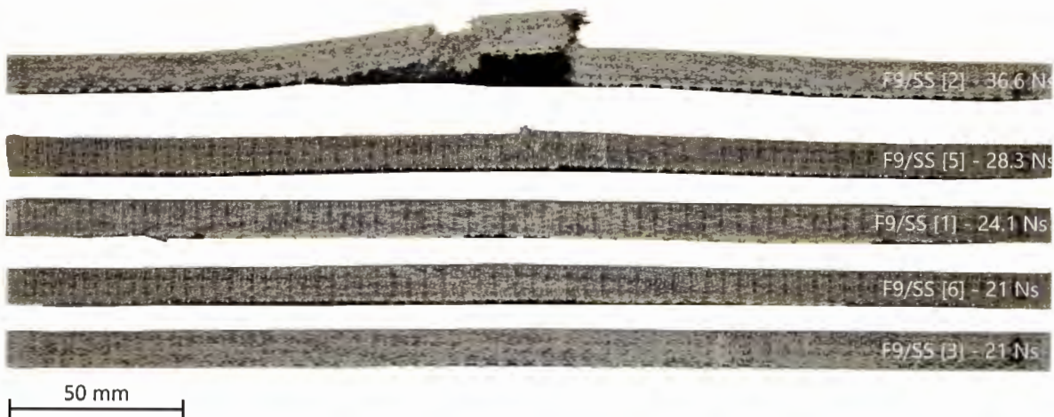
Figure 8-35: Cross section photographs for blast tested Flax 9/Super Sap panels
