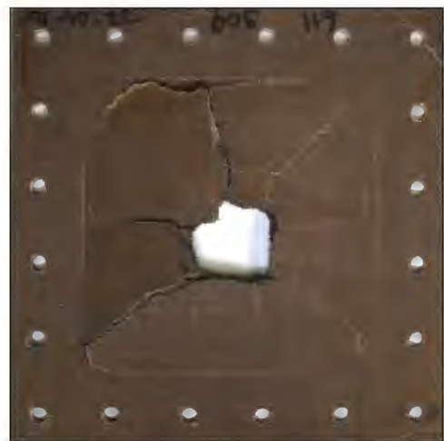
Figure F-2: Front and back surfaces of different blast tested Jute 13/Super Sap panels subjected to an impulse above 19.5 Ns (with no crack tracings)
