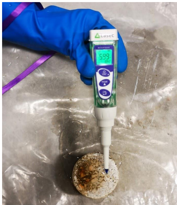
Figure 3.8: Surface pH measurement on an exposed concrete specimen
