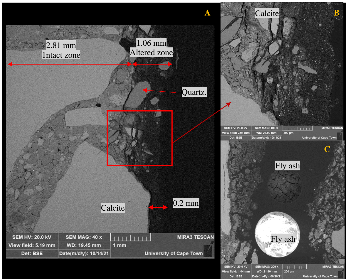
Figure 5.10: SEM-BSE image for SRPC+FA concrete after two years of exposure at NAS M19
