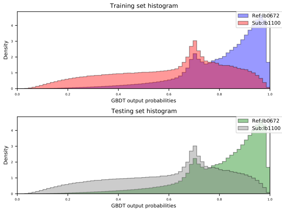
Figure 7.16: GBDT output probability histogram as a density plot (area under the curve normalised to 1) for LB 1100 (2 835 968 tracks).
