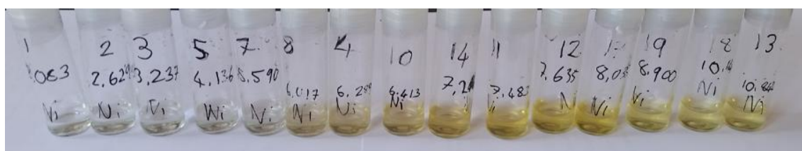
Figure 4.1: Visual observation of the colour change during a pH increase from 2-10, in increments of 0.5 from left to right for the copper(II) complexes, (a)(i) Cu-GLH, (a)(ii) Cu-Sar-LH, (a)(iii) Cu-GFH and (a)(iv) Cu-Sar-FH, as well as for the nickel(II) complexes (b)(i) Ni-GLH, (b)(ii) Ni-Sar-LH, (b)(iii) Ni-GFH and (b)(iv) Ni-Sar-FH.
