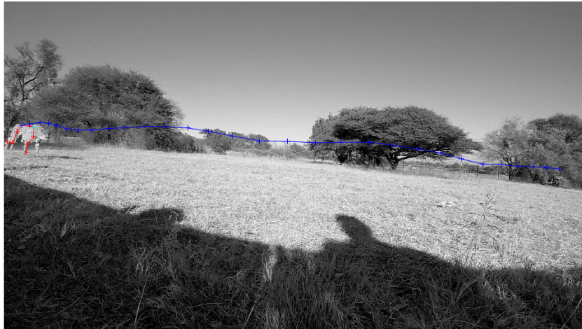
Figure 42: The progression of the estimated reference joint trajectory (blue) in the image plane. Note its approximately sinusoidal path of about 3Hz , confirming the assumed three gait motion of the subject.
