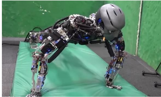
Figure 74: The Kengoro humanoid robot with intricate musculo-skeletal links (Image credit: JSK Laboratory, University of Tokyo).
