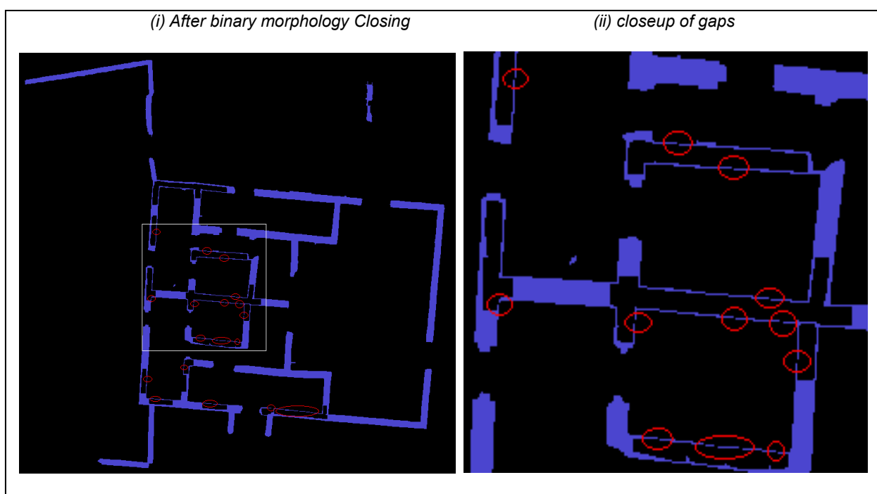
Figure 16: Example of cross-section profile with gaps
