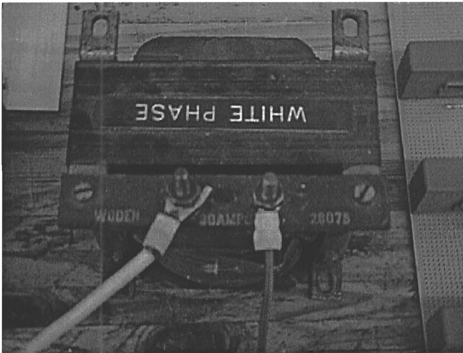
Inductance used in the experiments
