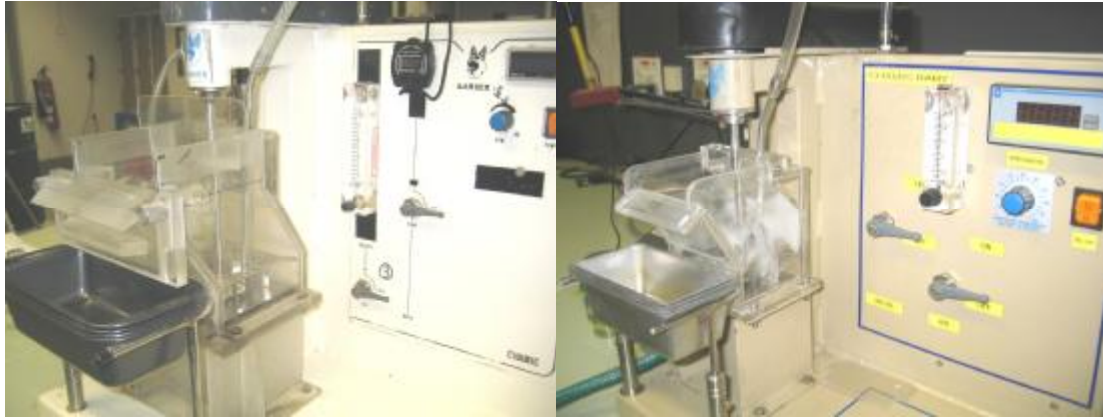
Figure 3.4: Modified Leeds flotation cells used during this study (the 3 l cell on the left and the 650 ml cell on the right)
