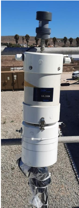
Figure 17: The MiniVol™ Ver 4.2 by Air Metrics installed at the Saldanha AQM Station
