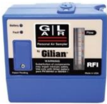
Figure 18: The Gilian GilAir-3 Sampling Pump (inteccon.inc, n.d.)
