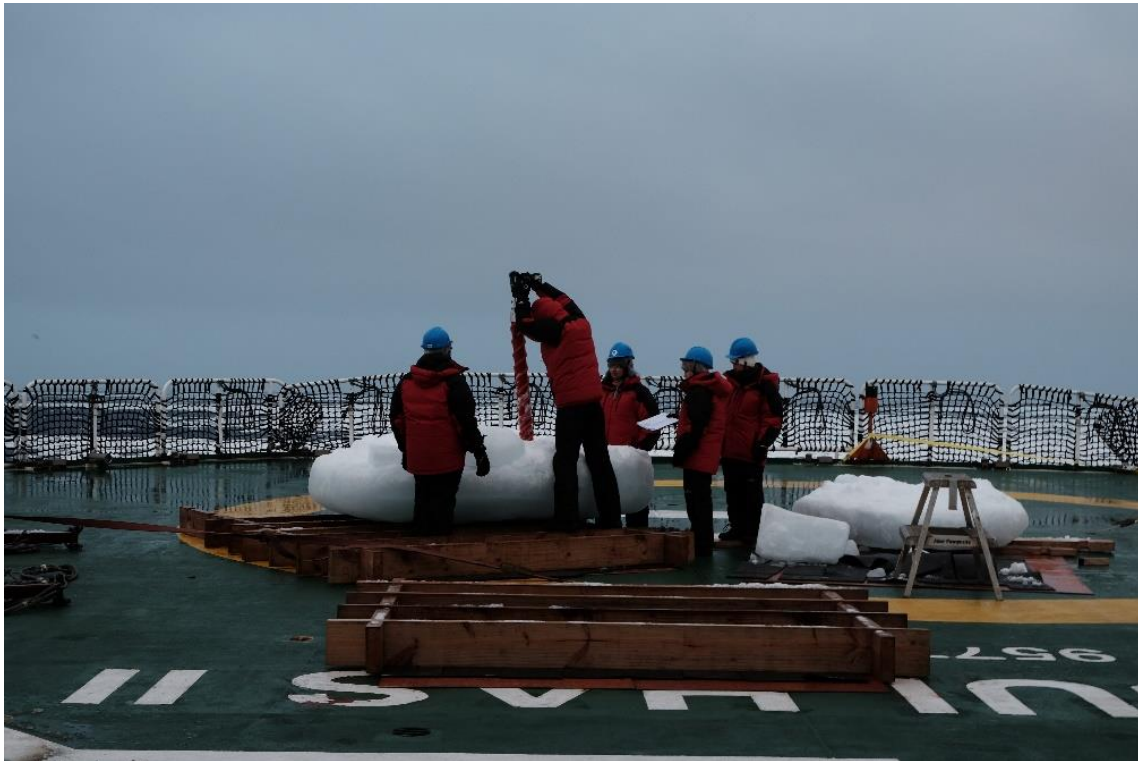
Figure A. 1: On deck coring of pancake
