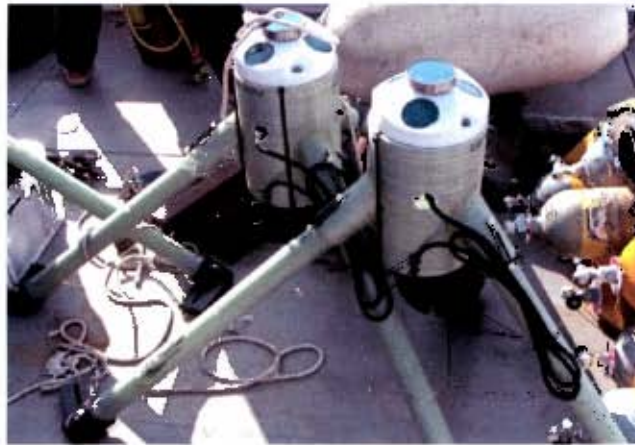
Figure 13: ADCPs and plastic frame
