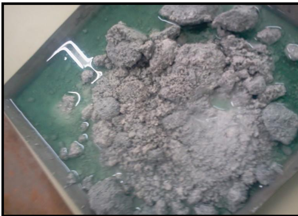
FIGURE 28: IMAGE OF A BAKED SAMPLE THAT ABSORBED MOISTURE FROM SURROUNDINGS.
