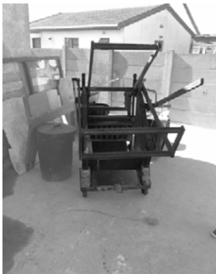
[50] Concrete block hand-press used to produce 6 blocks at a time, a total of 1000 blocks can be produced in a day.
