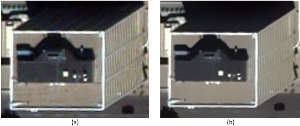
Figure 37: The results of a bilateral filter on satellite image data. The salt and pepper effects in image (a) are smoothed out with all edges preserved in image (b).
