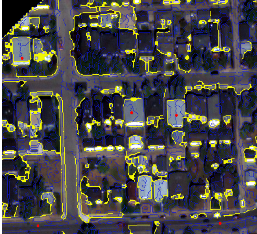
Figure 83: Comparison of ABED (blue) and Canny (yellow) in a residential area. ABED over-detects small objects such as trees. However, ABED partially detects gable roof ridge lines that were not detected by Canny edge detection, shown by the red dots, ABED recovers most of the missed roads and captures boundaries missed by Canny on some houses. This level of detail that is missed by canny results in incomplete building form, while ABED detects edges representing form and detail. This shows the advantages of automated parameter tuning over thresholding.
