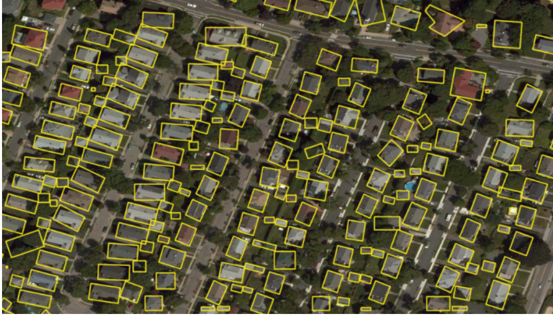
Figure 18: Building footprints derived from deep learning [171]. Some of the footprints shapes do not match the building shape and orientation.
