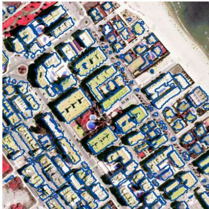
Figure 16: Object detection using satellite images [43]. Building object extents are shown in blue. often the result of filtering and object detection algorithms are object extents.
