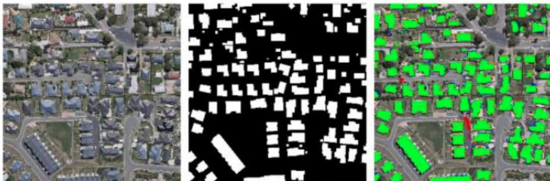
Figure 10: Sample results from deep learning presented by Li et al. [149] showing how object extents are detected. First column is the input image, second column represents ground truth. Green in the third column are correctly segmented building and red shows wrong detections.
