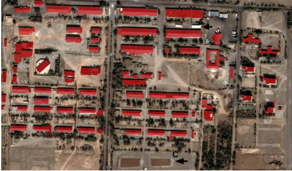
Figure 9: Building detection results on a high resolution image. The red areas indicate the extents of the buildings detected by Attarzadeh and Momeni [146].
