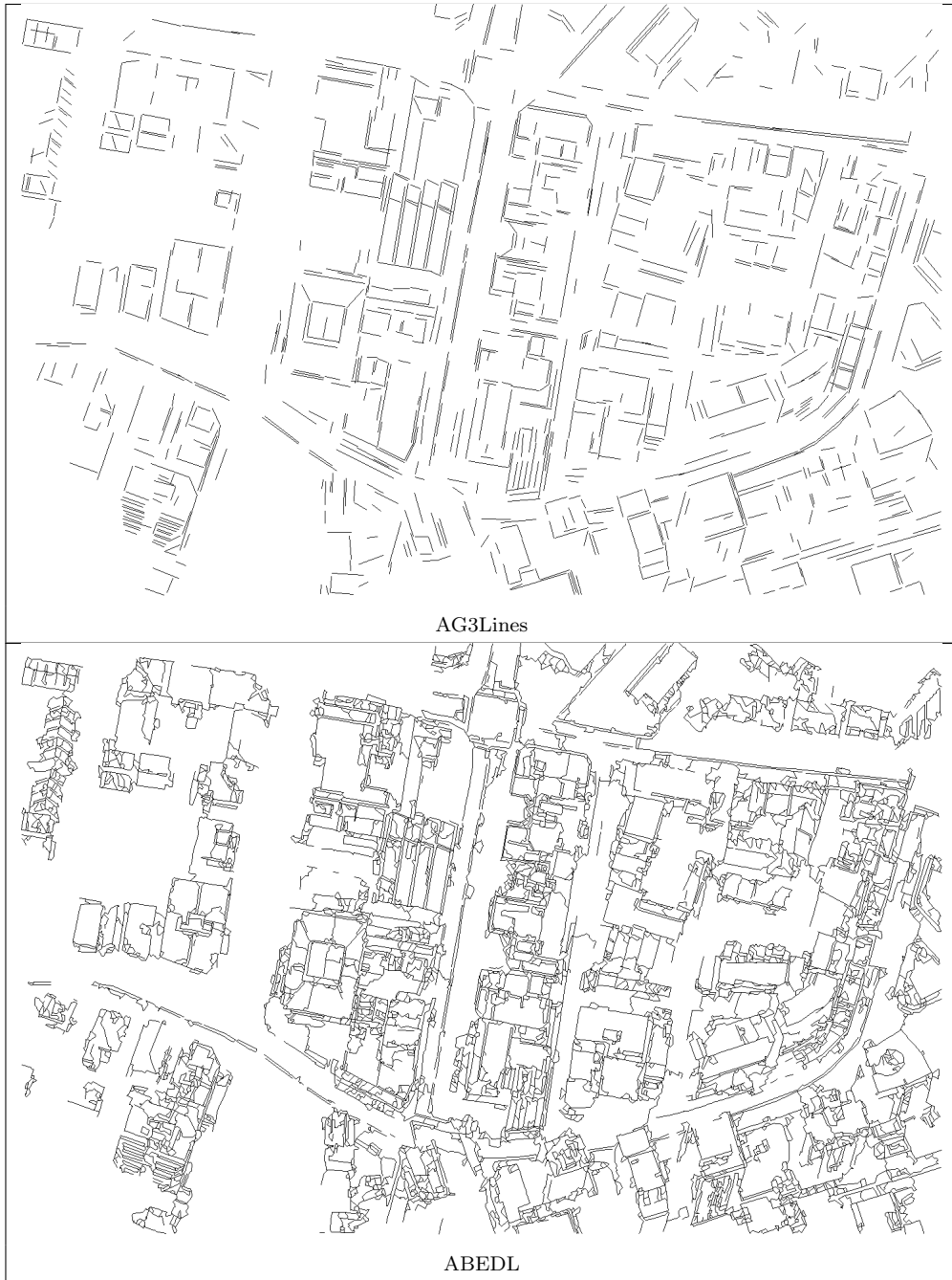
Figure 120: Boundary detection results comparison for Brisbane CBD ( TI_1 ). ABEDL, has denser and longer lines. Links which connect valid lines have been retained to preserve object detail that improves wireframe results.
