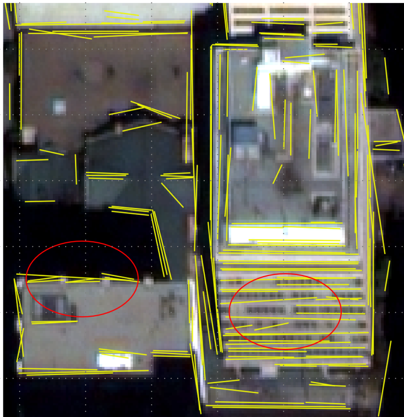
Figure 50: Errors introduced as a result of line fitting. Edges circled in red show random rotation when compared to the expected direction. Edges in the image above were recovered using EDLines.
