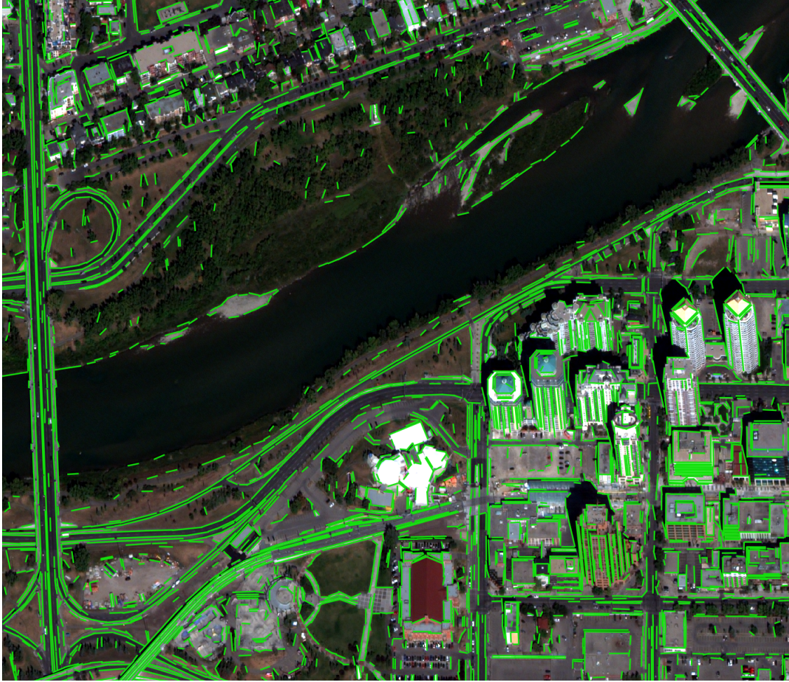
Figure 7: Results of Line Segment Detector (LSD) [4] on a satellite image. This is an example of line features extracted from a satellite image. The lines are characterised by fragmentation and some lines are missing.
