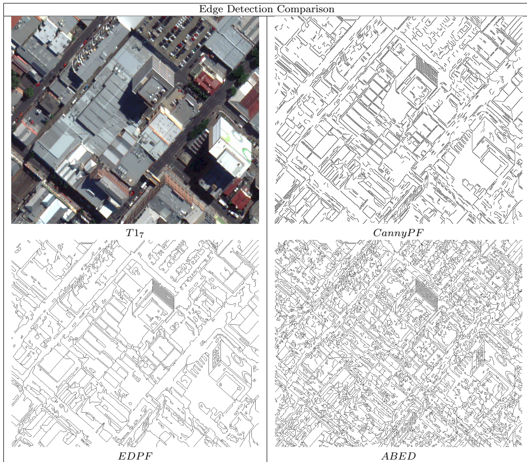
Figure 77: Edge detection results comparison of ABED versus CannyPF and EDPF for Brisbane, image T17 . ABEDL, has denser edges in the bottom right image in comparison to the other detectors in a CBD area with reduced fragmentation
