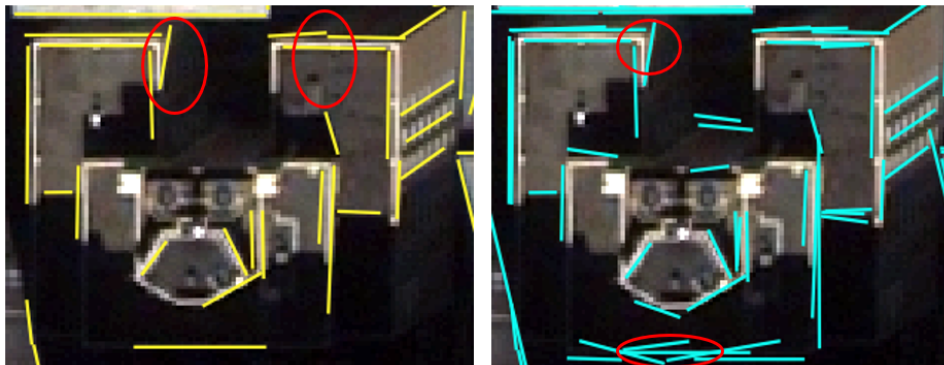
Figure 49: Errors introduced as a result of line fitting. While all roof edges are supposed to be perpendicular, some rotations can be seen with some of the edges, resulting in non-parallel and non-perpendicular edges circled in red. Edges in the left image were recovered using LSD and the second set of edges on the right were recovered with EDLines.
