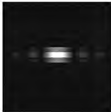
Figure 3.7: Magnitude of the focused target in the image domain focused to 20.5 m in azimuth (Simulation A).
