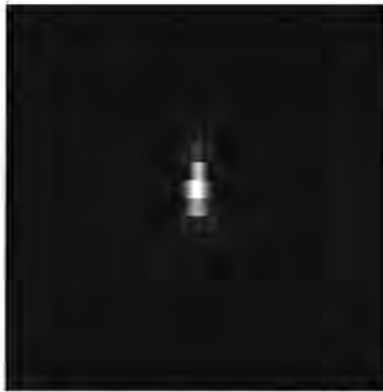
Figure 3.11: Magnitude of the focused target in the image domain focused to 3.1 m in azimuth (Simulation A). A Hamming window has been applied to the azimuth matched filter in the signal domain.
