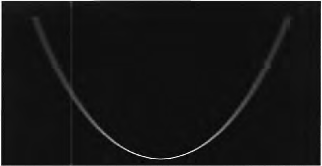
Figure 3.4: The magnitude of the simulation signal after the azimuth Fourier transform with zero Doppler frequency centred (Simulation A). The full azimuth sampling bandwidth of 250 Hz is represented by the horizontal dimension and slant range increases vertically (528 samples full image extent). The dispersion in azimuth at Doppler frequencies away from zero is clear.
