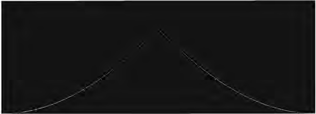
Figure 4.2: The magnitude of the 30 km reference function, cyclically shifted so that the zero Doppler point lies at the origin. Azimuth extent (horizontal) is 29811 m and range extent (vertical) is 4400 m.
