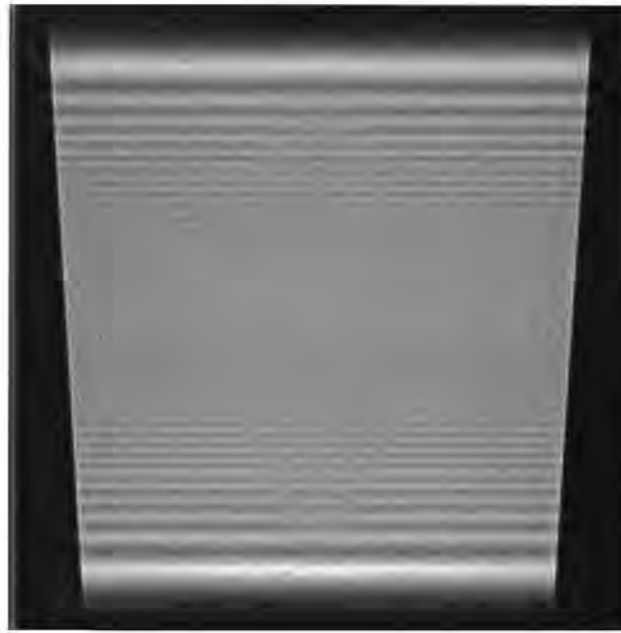
Figure 4.3: The magnitude of the 30 km reference function in the 2-D frequency domain (as input to Step E), zero-centred in both dimensions. Full image azimuth frequency extent (horizontal) is 250 Hz, full range frequency extent (vertical) is 22 MHz.
