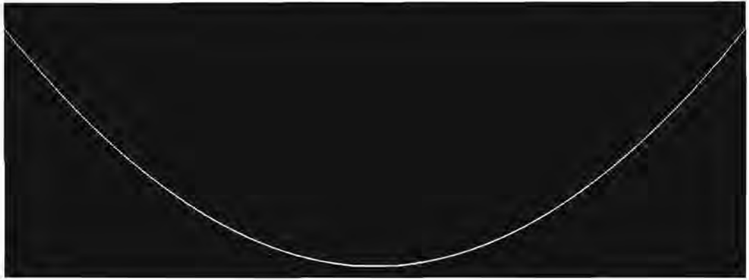
Figure 2.5: The magnitude of a range compressed SAR simulation signal in the slant range image, azimuth signal domain. The slant range resolution is 9.74 m. The full image azimuth extent is 27.979 km (horizontal) and slant range extent is 3.600 km (range increases vertically). The simulation is over a 50 degree azimuth extent for a target at 30 km closest approach range.
