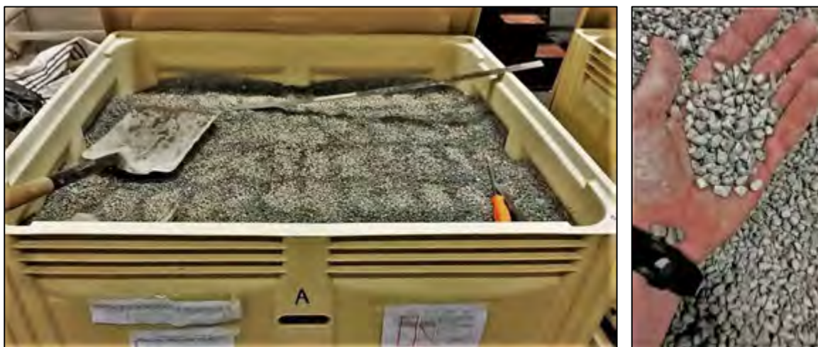
Figure 4-20: Early stages of the excavation of Pavement A where large amounts of ‘dust’ were found adhering to the bedding gravel
