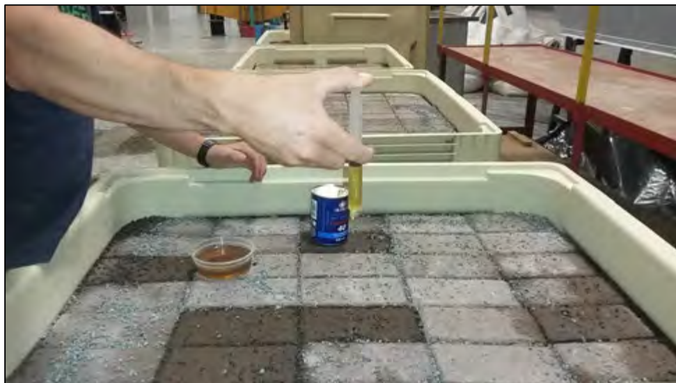
Figure 3-10: Oil application to laboratory pavement surfaces
