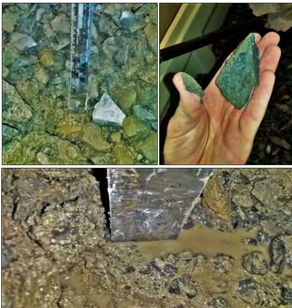
Figure 4-26: Sediment observed at different depths within Pavement D
