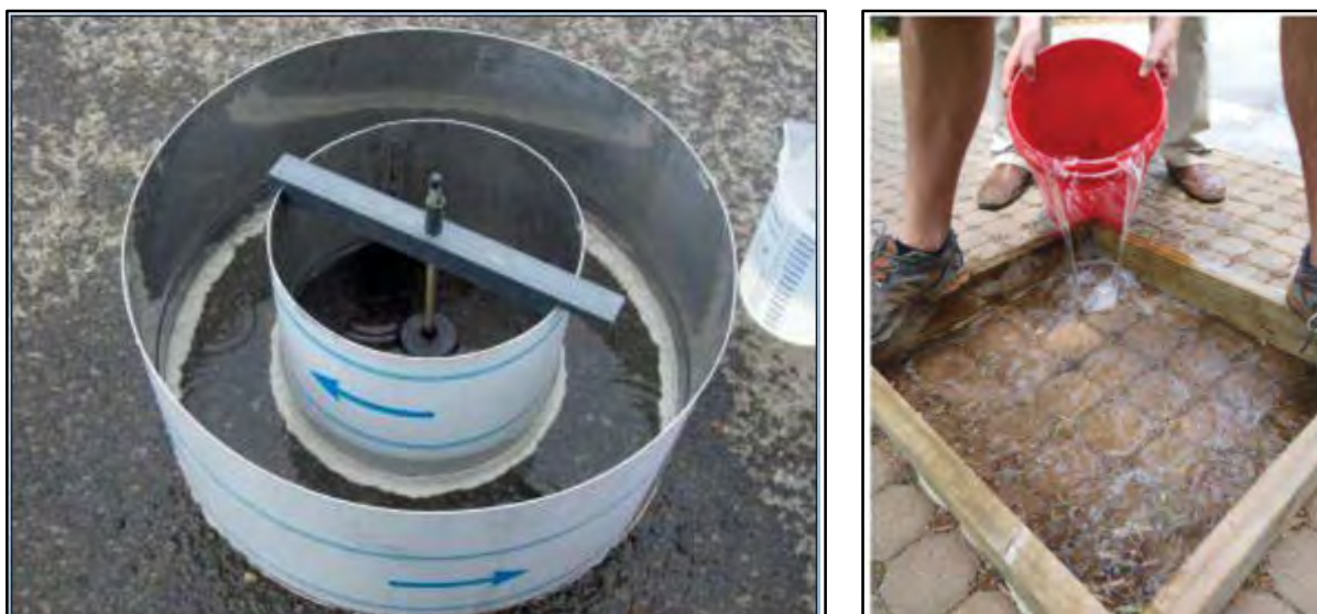
Figure 2-12: Double-ring infiltrometer (left); Simple infiltration test (right) (Bean et al. , 2004)
