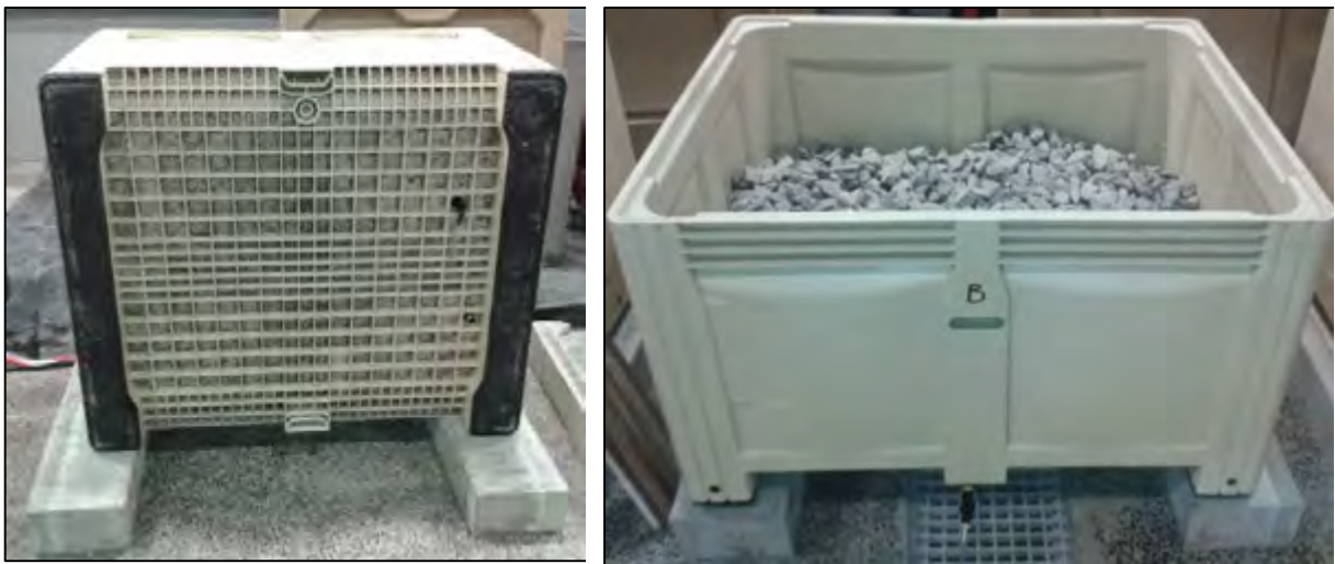
Figure 3-2: Bins positioned on concrete blocks to accommodate drainage tray
