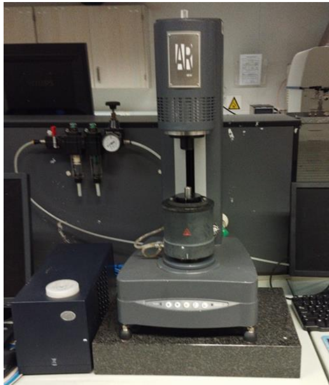
Figure 3-6: AR1500EX-TA rheometer fitted with a standard vaned rotor geometry.
