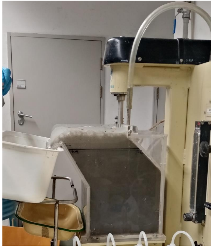
Figure 3-4: 8 L Leeds batch flotation cell.
