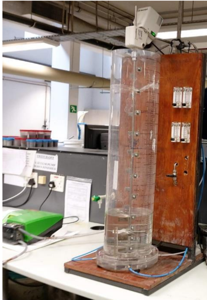
Figure 3-5: Column used to investigate the effect of oil on the froth stability of the normal and altered ore.
