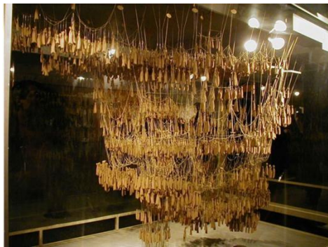
Figure 9. Catenary form modeling by Antonio Gaudi. 36. ITA Project. Antonio Gaudi, Sagrada Familia, Barcelona – Spain 1883- (unfinished). [Online] Available from http://www.itaproject.eu/TTU/6/sagrada.html [Accessed April 2015]
