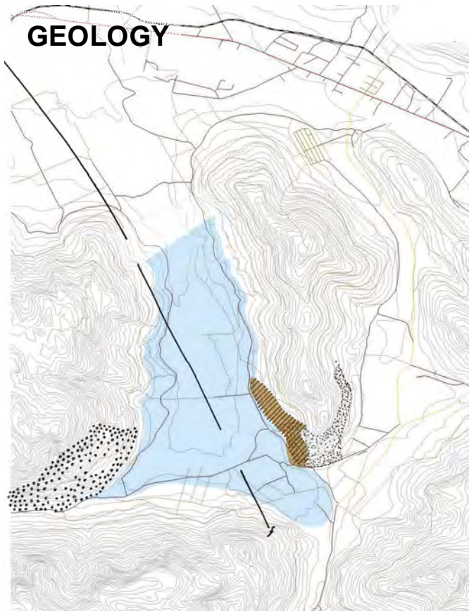
Klipheuvel layers result in Rock Falls
