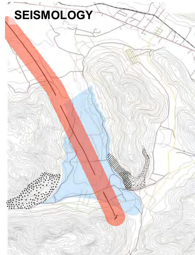
Regional Fault Line through the Dam site
