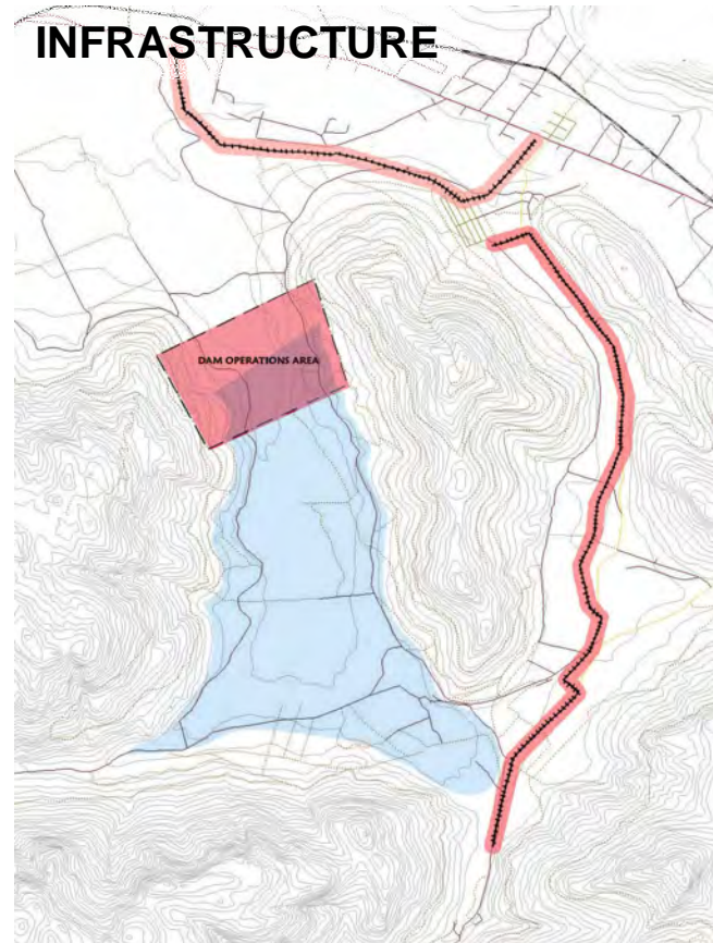
A setback of 30m is necessary from existing powerlines. These also pose as a visual constraint for development.
