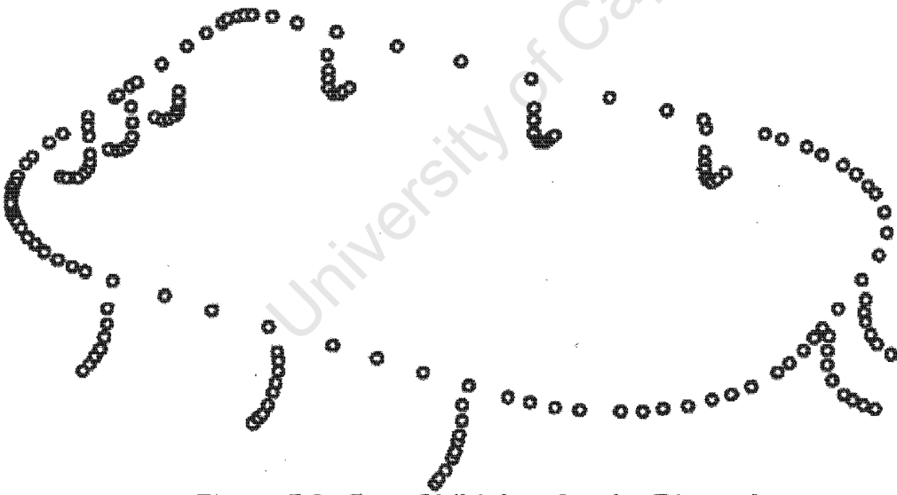
Figure 5.2 : Raw CMM data for the Die tool
