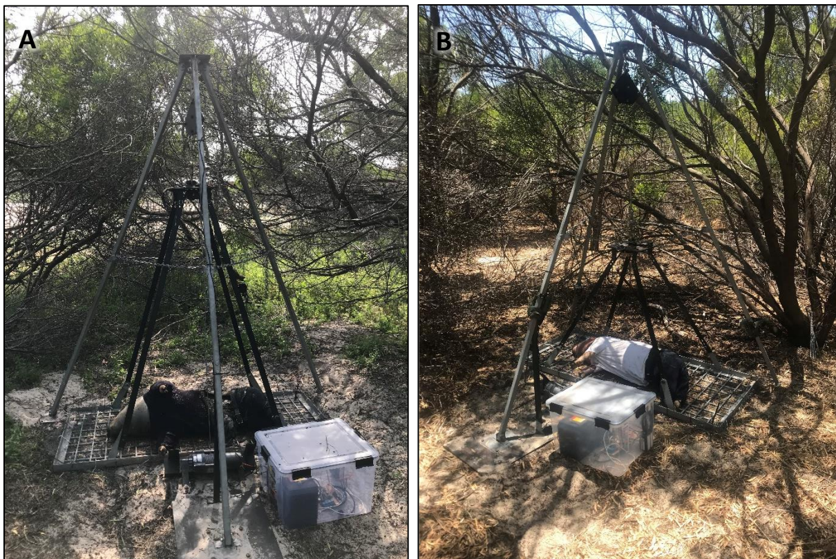
Figure 2.7: Equipment used for weight loss and scavenger monitoring in cycles 3 and 4. A) Prototype automated weighing apparatus (09/2019) consisting of a 12V battery-powered winch, a pulley system attached to the steel tripod, and a sub-frame mounted above the weighing grid, used in cycle 3. B) Version 2 (01/2020) of the automated weighing system with a shorter sub-frame, wide-angle camera, and improvements to the code used in cycle 4 (Finaughty et al., 2020, 2021).
