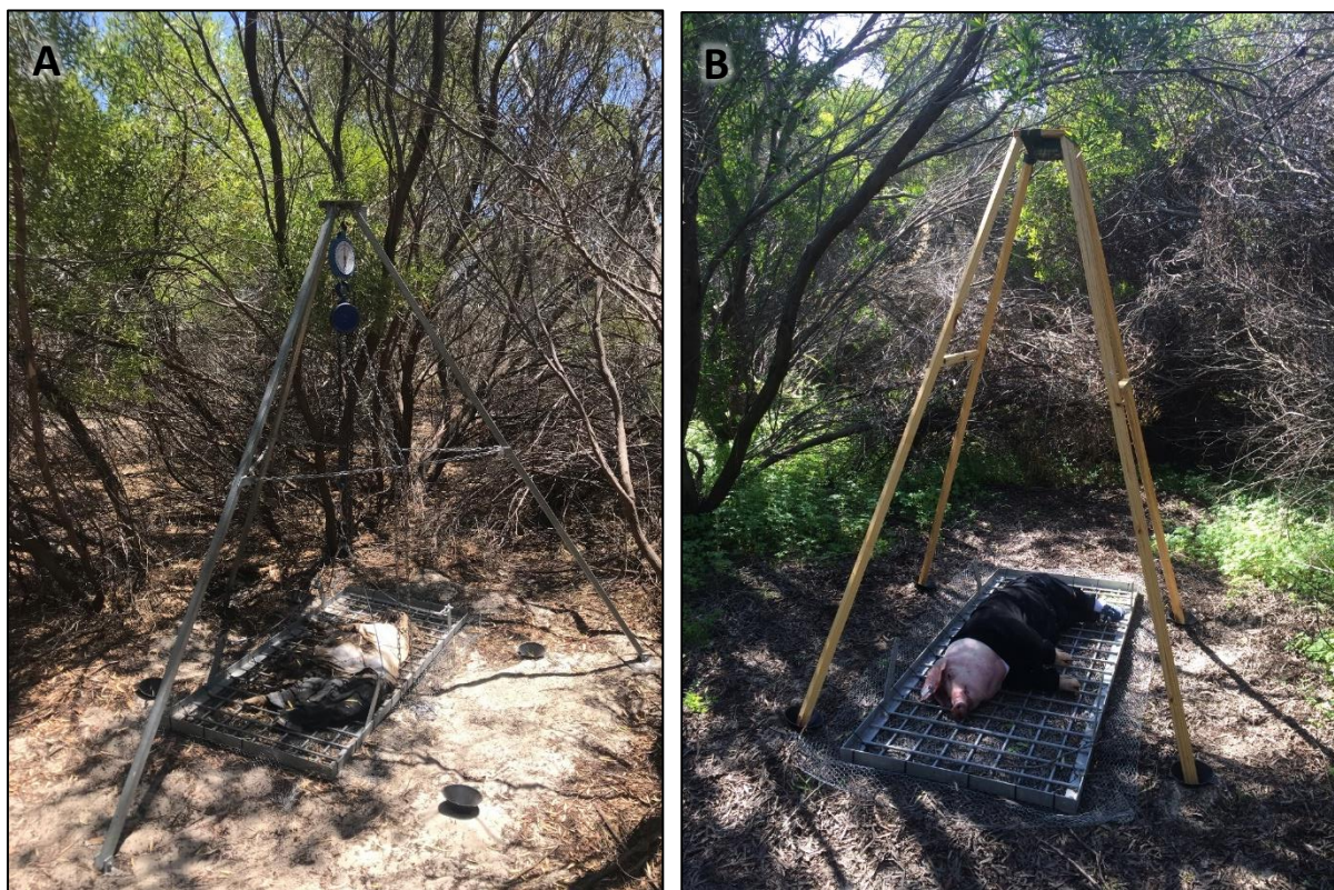
Figure 2.6: Equipment used for weight loss and scavenger monitoring in cycles 1 and 2. A) The steel tripod with a block and tackle system used to lift the carcasses and grid (1 x 2 m) to take daily weight readings from an analogue scale in cycles 1 and 2. B) The wooden four-legged structure used to mount the motion-activated cameras directly above each carcass in cycles 1 and 2.
