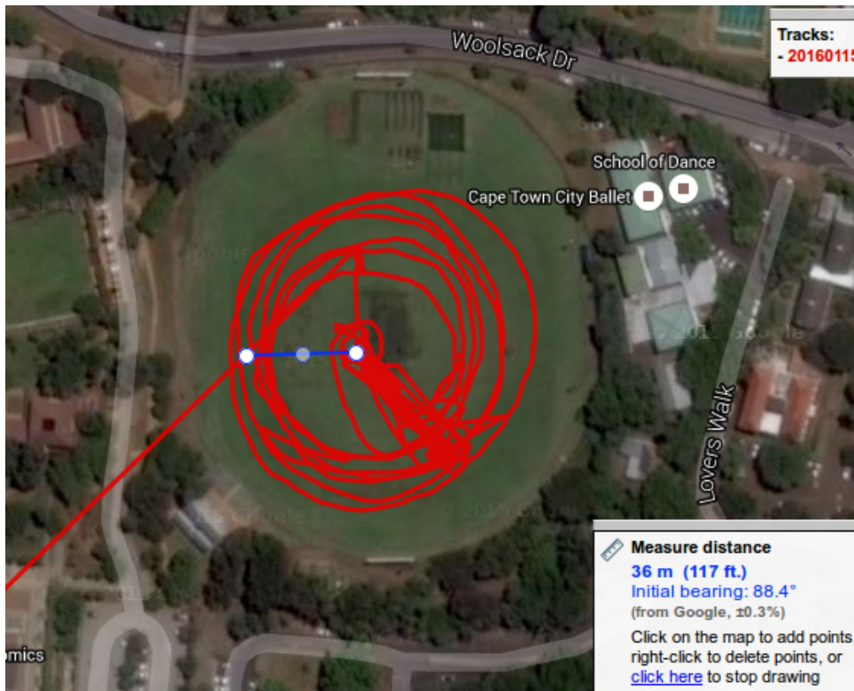
Figure 7.7: Route of the person walking with the transmitters during the field trials, according to GPS logger. The curve is a smoothed collection of timestamped lat/long coordinates
