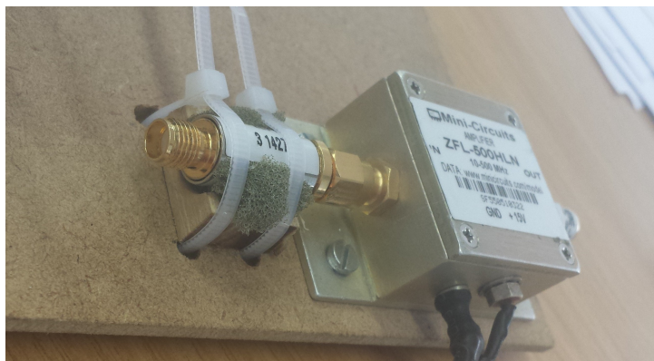
(c) Close up of a low pass filter connected to an amplifier, held down to make it more rugged in the field.
