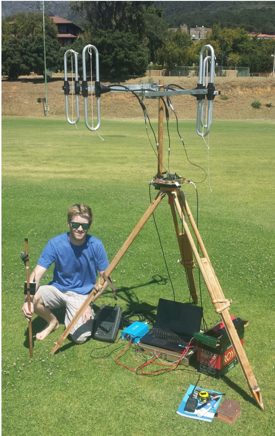
Figure 7.5: Setup on UCT sports field focused on receiver and front end. From top to bottom: four element antenna array, SMA cables into RF front end board, cables into ROACH (shiny box under the laptop). ROACH running directly off of 12 V battery, with the battery in the red and black box (right). Blue inverter for charging laptop between tests. Grey box on the left is R&S spectrum analyser for checking the power level coming out of the LNAs before connecting to ROACH ADCs.
