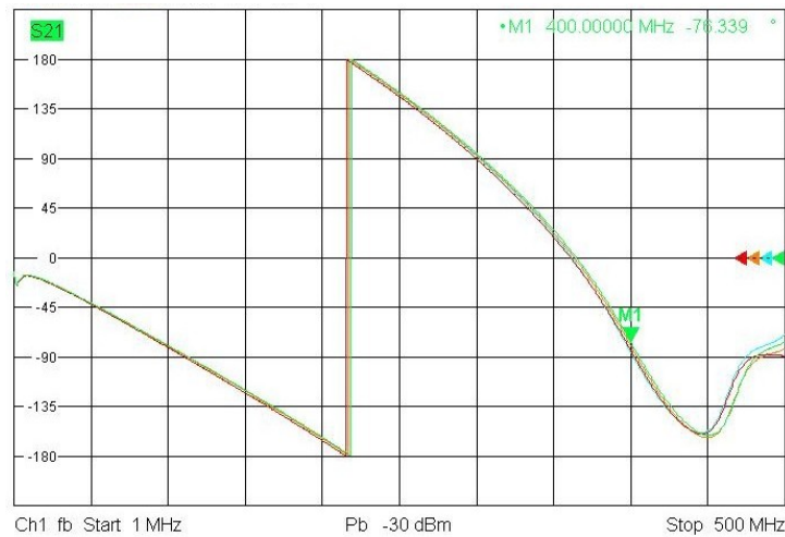
(c) Phase from 0 to 500 MHz showing very good phase matching over operating frequency range below 350 MHz
