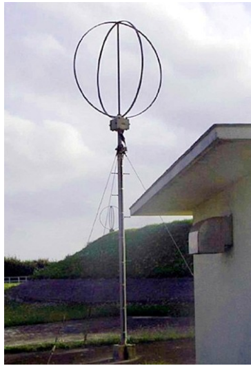
(a) Example of crossed loop antenna.
