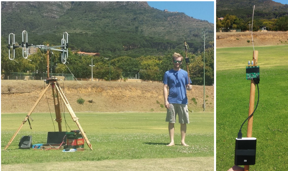
Figure 7.6: Photo on UCT sports field (left) showing how the transmitter was carried around, with both it and the receiving antennas at a height of approximately 2 m. The PCB in (right) is the Valon synthesiser. The shield of the USB cable going down and the wire coming out of the SMA port pointing up act as a quarter-wave dipole.
