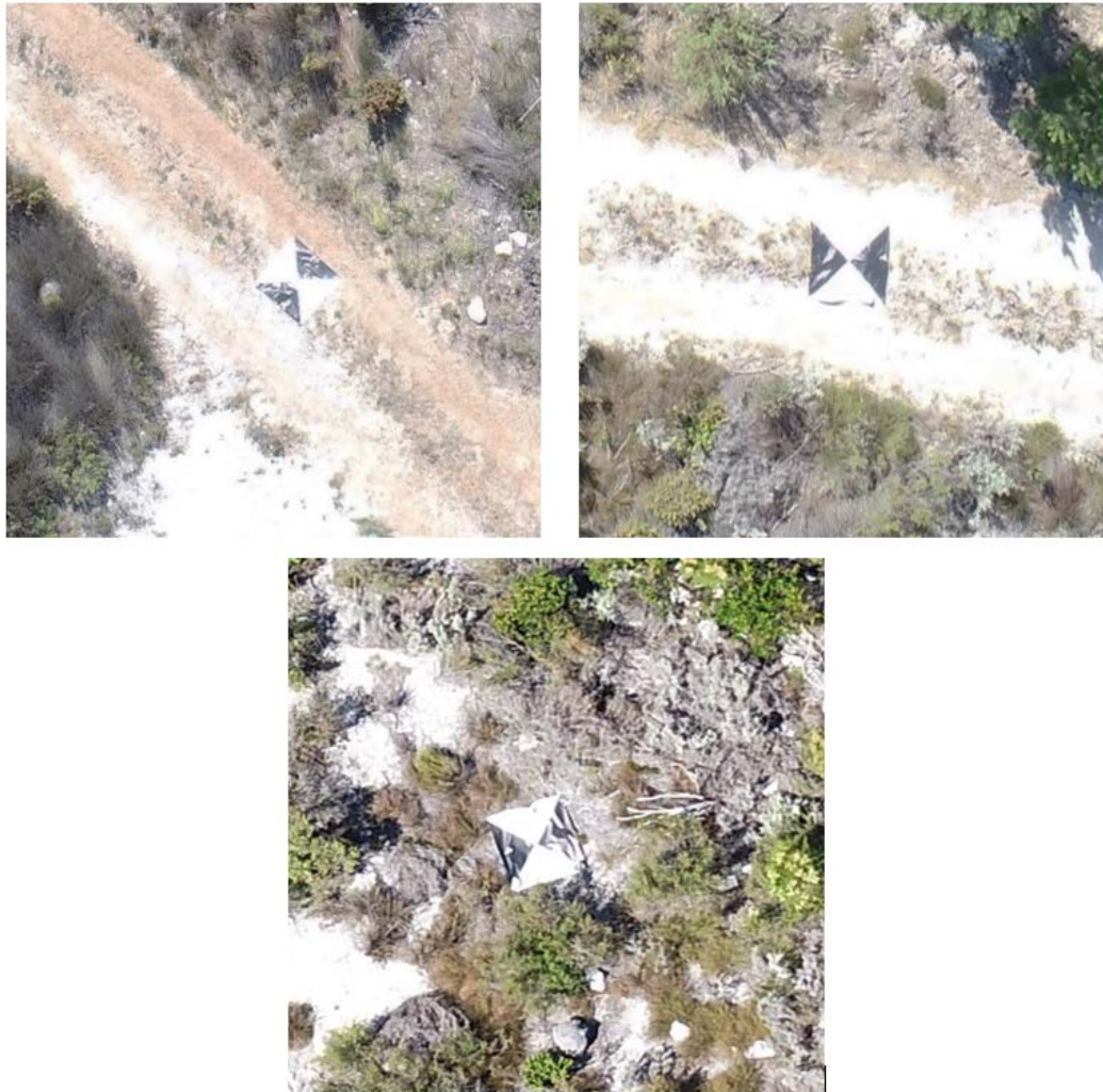
Figure 4.7 | (a) GCP1, (b) GCP2, (c) GCP4 – three of the four GCPs placed around H_{etero}FS_2
