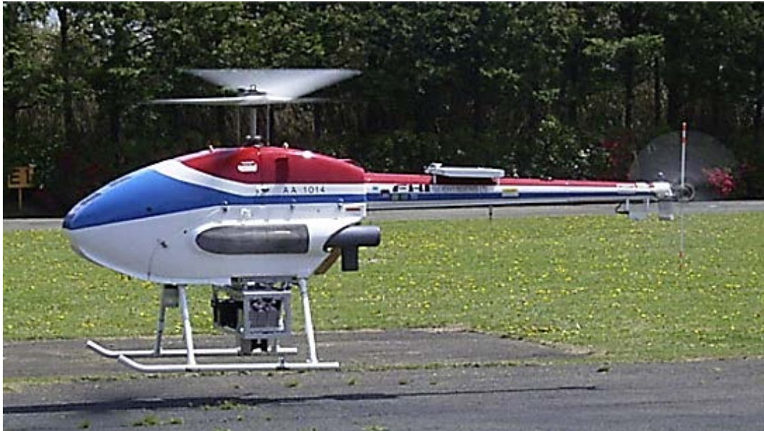
Figure 2.5 | Subaru RPH2 Multi-sensor model helicopter (Nagai et al., 2004)
