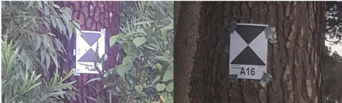
Figure 4.22 | Two of the 44 TLS targets taped to individual tree trunks and features at HeteroFS 1
