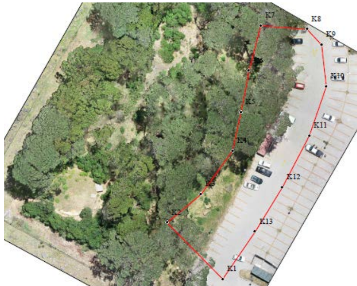
Figure 4.23 | Scan positions K1 to K13 (black dots) and the traverse (red line) of the TLS survey at H_{eteroFS_1}
