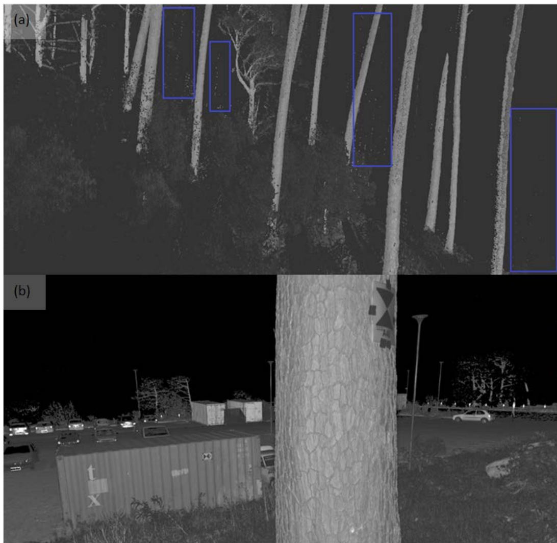
Figure 4.26 | (a) Erroneous points (in blue boxes) present in the dataset. These points are most likely a result of backscatter caused by heavy presence of dust in the area during scanning, (b) Structures present in the point cloud – cars, shipping containers, streetlamps – prior to being removed.
