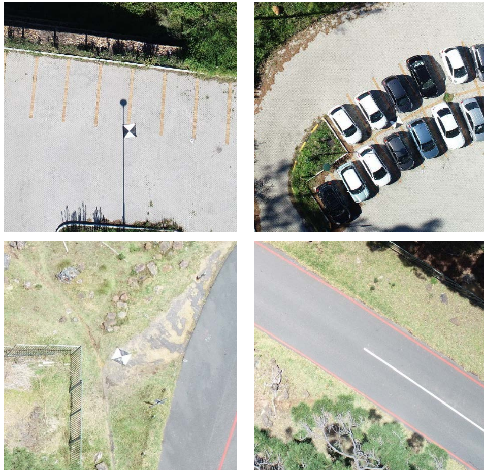
Figure 4.4 | (a) GCP3, (b) GCP2 (between cars), (c) FUJ, and (d) GCP1 – four of the six GCPs placed around H_{eteroFS_1}
