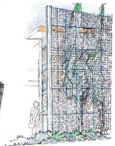
5m high Bekaert fence to restrict direct access yet allowing for visibility of the trees. The fence is uncuttable and unclimbable.
