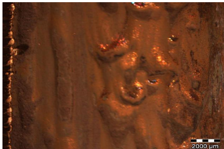
Figure 2.14: Erosion - complex profile of cavities.
