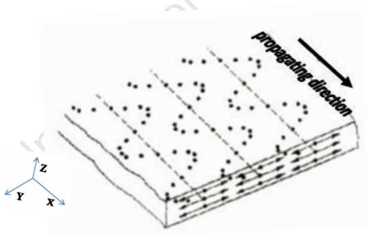
Figure 2.21: Wave propagation motion of SH modes. Particle motion is restricted to the y -direction only. Wave propagation is the x direction as shown [14].
