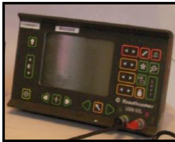
Figure 4.1: Conventional ultrasonic test set, USN52L.
