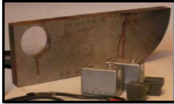
Figure 4.3: Calibration block, IIW-2, used for the calibration of the transducers.
