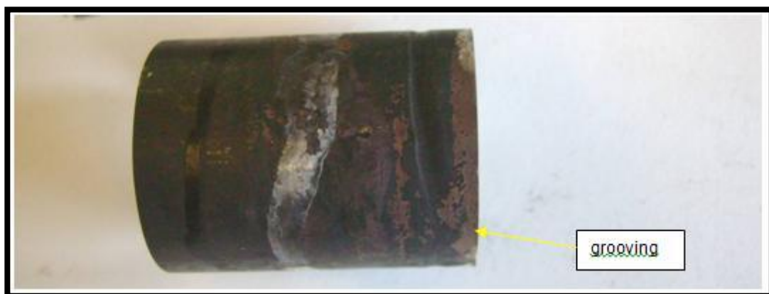
Figure 2.16: Ammonia grooving at a slight angle to the tube axis [18].
