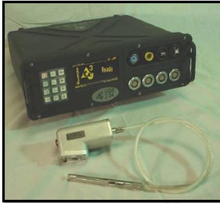
Figure 3.14: Guided Ultrasonics Limited Wavemaker G3 with in-bore transducer. It utilises PZT transducers and has 32 channels [90].
