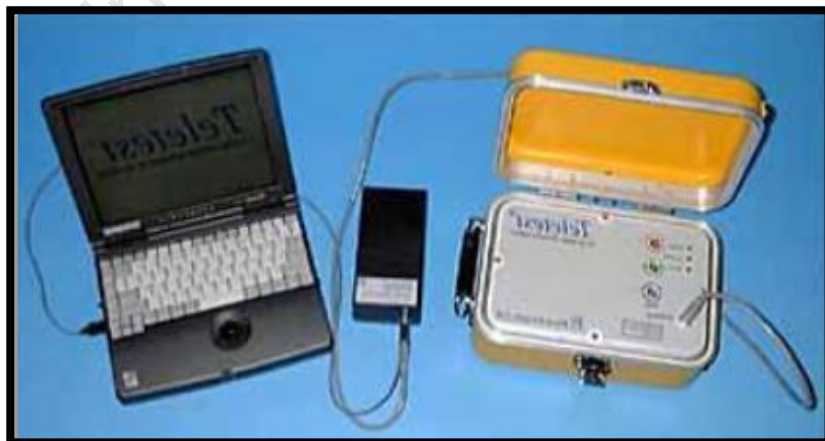
Figure 3.13: The Teletest test set supplied by Teletest and supported by TWI. It is based on PZT transducers and is designed to generate the L(0,2) and L(0,1) modes [89].
