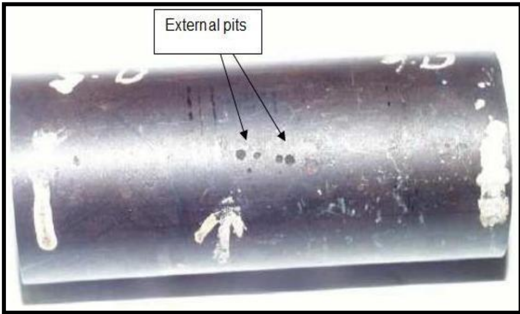
Figure 2.4: External pitting cluster in stainless steel tube [17].
