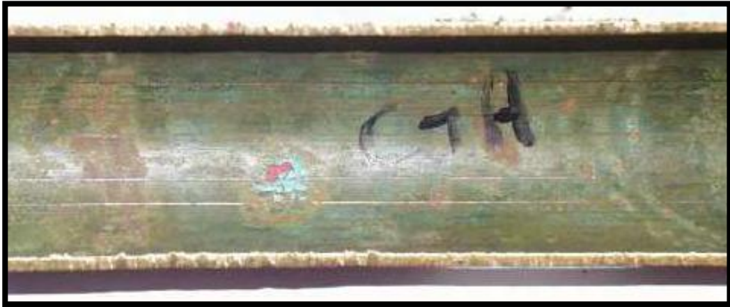
Figure 2.8: Isolated pit with asymmetrical shape [18].
