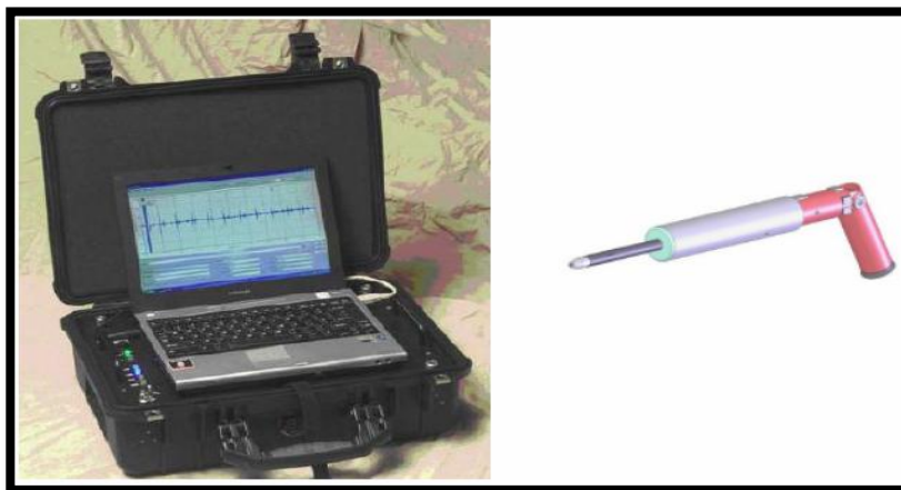
Figure 3.12: The MSsR3030R along with the in-bore transducer is developed by SwRI. It generates the T(0,1) mode and has a 250kHz bandwidth and 2 channels [88].
