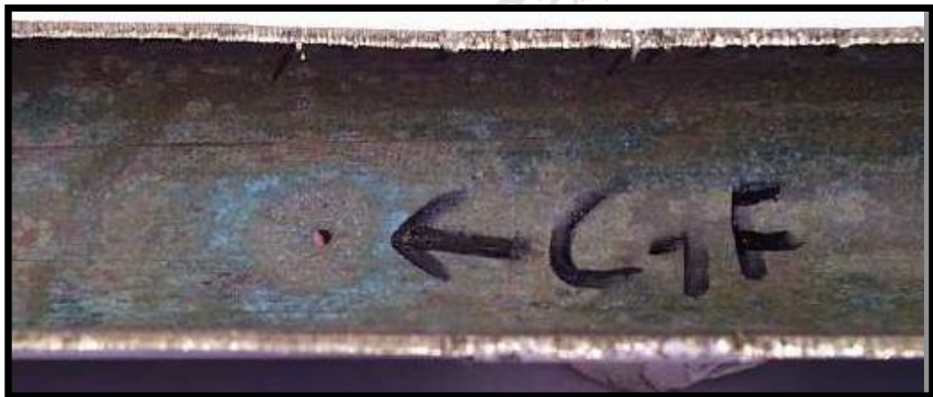
Figure 2.9: Isolated, symmetrical pit [17].
