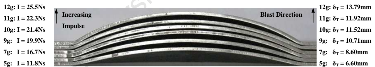
Figure 37: Photograph of the cross-sections of the target plates for a blockage ratio of 89%
