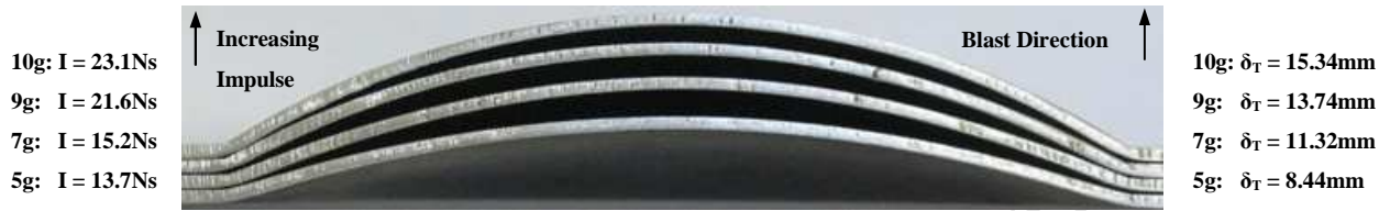
Figure 52: Photographs of the cross-sections of the target plates for a rigid perforated plate with blockage ratio of 75%
