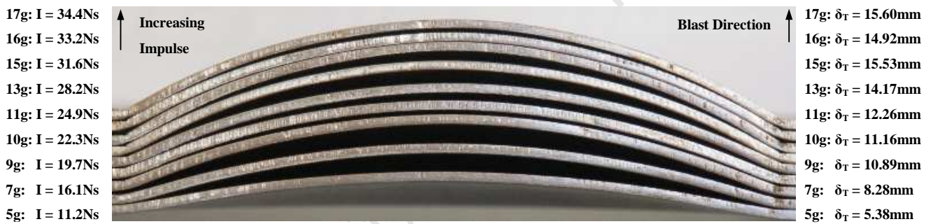
Figure 53: Photographs of the cross-sections of the target plates for a rigid perforated plate with blockage ratio of 89%
