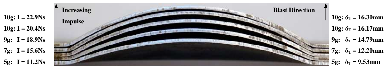
Figure 34: Photograph of the cross-sections of the target plates for a blockage ratio of 50%
