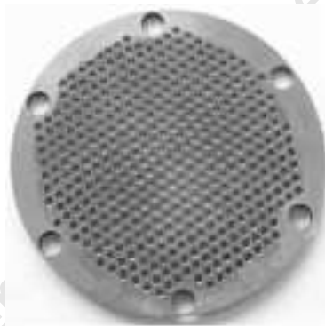
Figure 14: Photograph of a perforated plate used by Medvedev et al [28]
