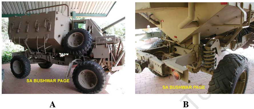
Figure 11: Photograph of the Buffel mine resistant infantry combat vehicle (A) and V-shaped armoured passenger compartment from the underside of the Buffel (B) [27]
