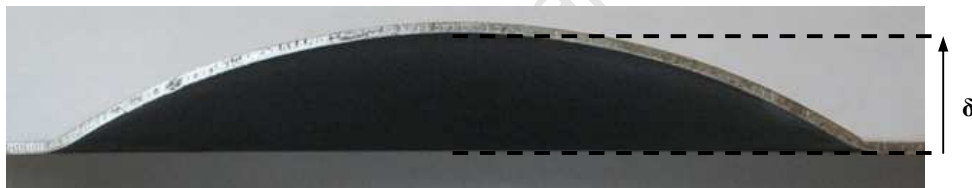
Figure 24: Photograph of target plate cross-section for test BR89R_15+1 ( I = 33.2\text{Ns} )
