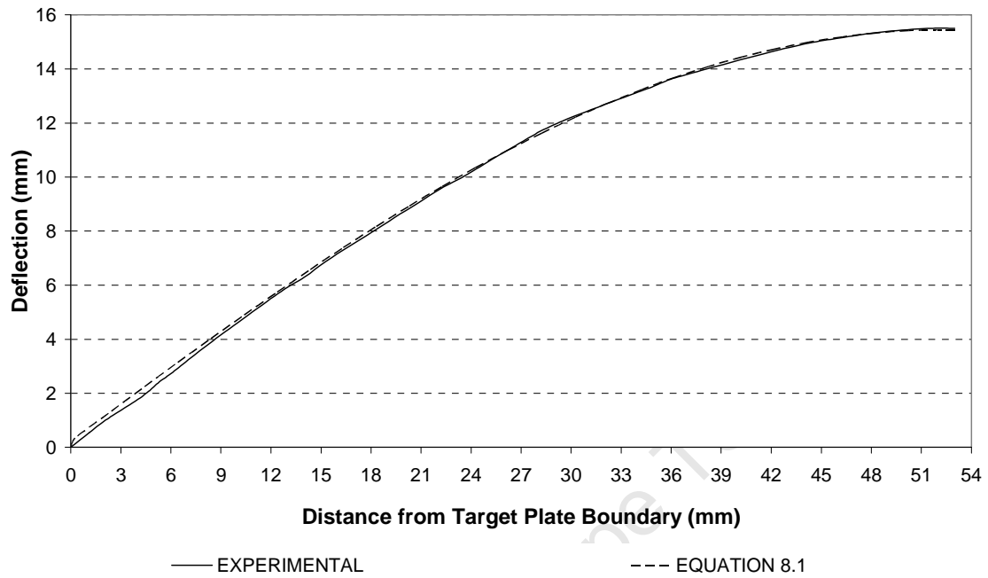
Figure 111: Graph of the experimental target plate profile and Duffey [41] shape function for a 9 gram charge mass and a blockage ratio of 25%
