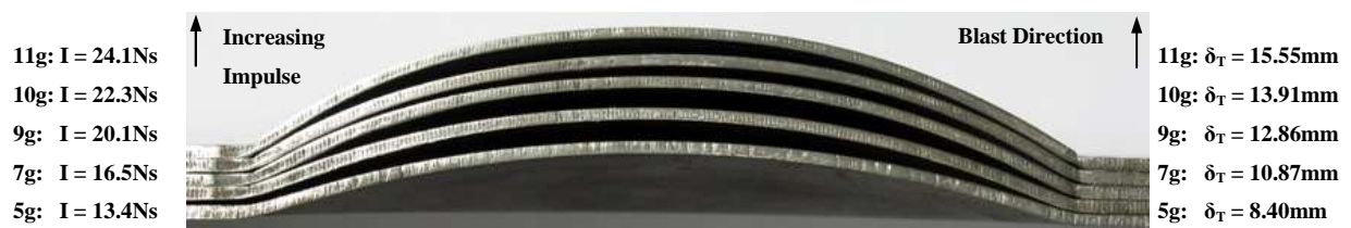
Figure 36: Photograph of the cross-sections of the target plates for a blockage ratio of 75%
