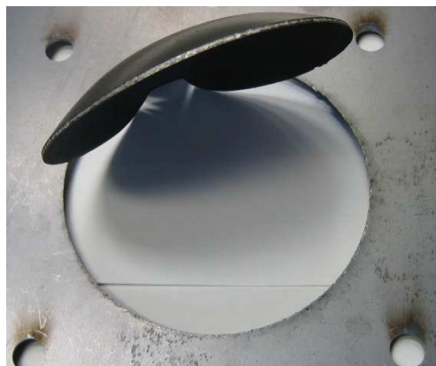
Figure 27: Photo graph of partial tearing at the boundary of the target plate for test BR65D_9+1 (I = 20.0Ns)
