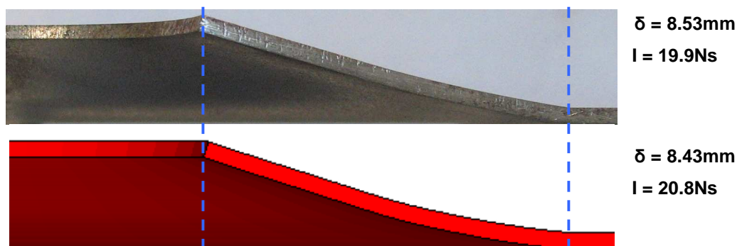
Figure 77: Perforated plate cross-sections for a 9 gram charge mass and a blockage ratio of 89%
