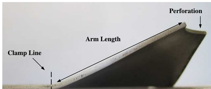
Figure 25: Photograph of perforated plate cross-section for test BR96D_14+1 ( I = 30.9\text{Ns} )
