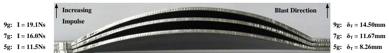
Figure 35: Photograph of the cross-sections of the target plates for a blockage ratio of 65%
