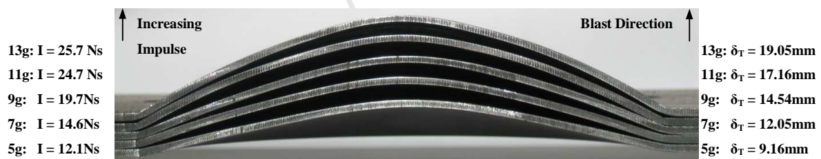
Figure 32: Photograph of the cross-sections of the target plates for the baseline blockage ratio of 0%
