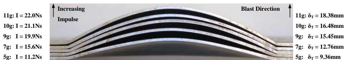
Figure 33: Photograph of the cross-sections of the target plates for a blockage ratio of 25%
