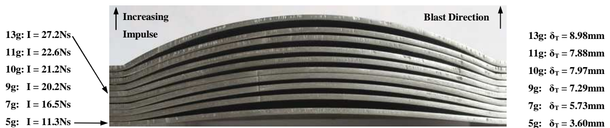
Figure 38: Photograph of the cross-sections of the target plates for a blockage ratio of 96%
